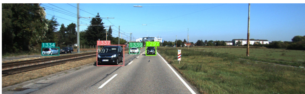
(b) The model incorrectly assumes parked car is moving
