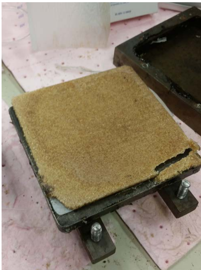
Figure 10. Resin wafer made of cation resin, anion resin, sugar, and polyethylene. The sugar is dissolved in a DI water soak for 24h prior to using the wafer in operation, allowing pores to form for solution to pass and aid in ion exchange.
