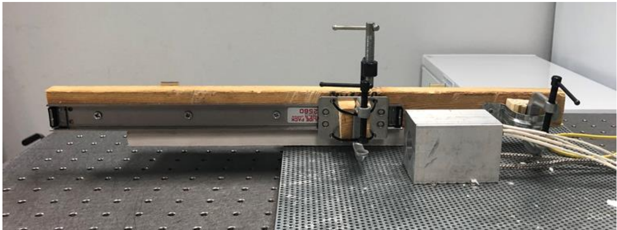
Figure 6. Device constructed to stretch larger diameter tubing to obtain tapered ends.
