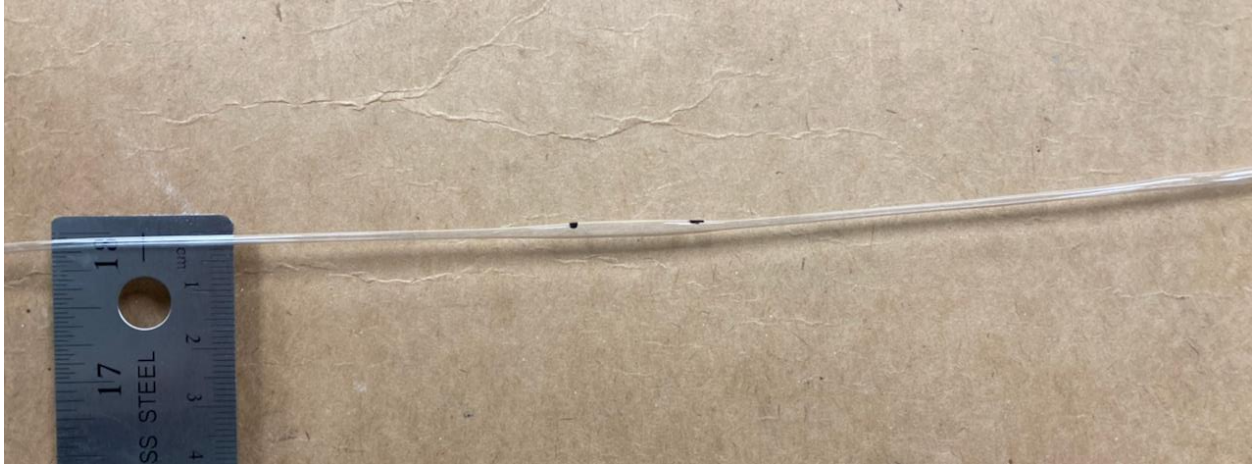
Figure 7. One of the parison preforms after being stretched in the necking device. The area between the two black markings is the original tubing diameter 2.73 mm and the outside tubing has a diameter of approximately 1.54 mm.
