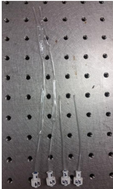
Figure 4. Results of temperature testing with fixed pressure and heat time. From left to right, temperatures are 90°C, 100°C, 110°C, and 120°C.
