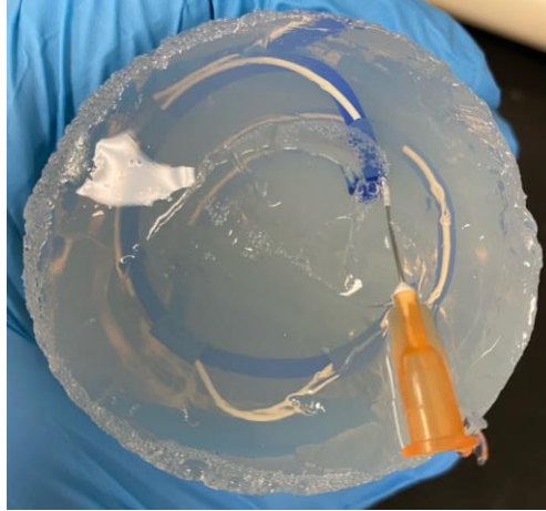
Figure 7. TPU and microporous membrane in gelatin clot analog with no apparent expansion after injecting fluid.
