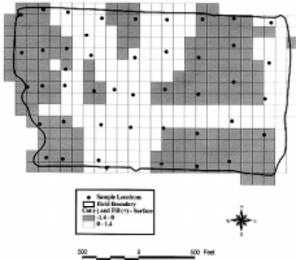
Fig. 3. Map of cut sheet used for land leveling. Positive values refer to areas of fill (ft) while negative values refer to areas of removal (ft). Data furnished by BOWLS Surveying, England, Arkansas.
