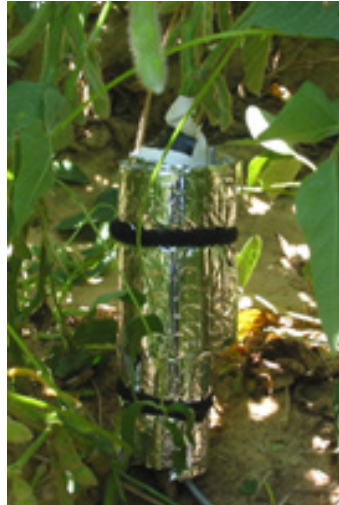
Fig. 2. Installation of sap flow sensor in soybean plant stem.
