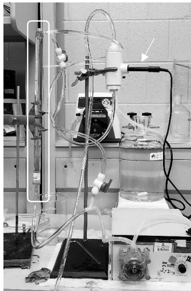
Figure 12: Equipment configuration for Membrane II. Membrane cartridge containing silver concentrate is circled. Downstream silver concentration measured with online conductivity probe (arrow).
