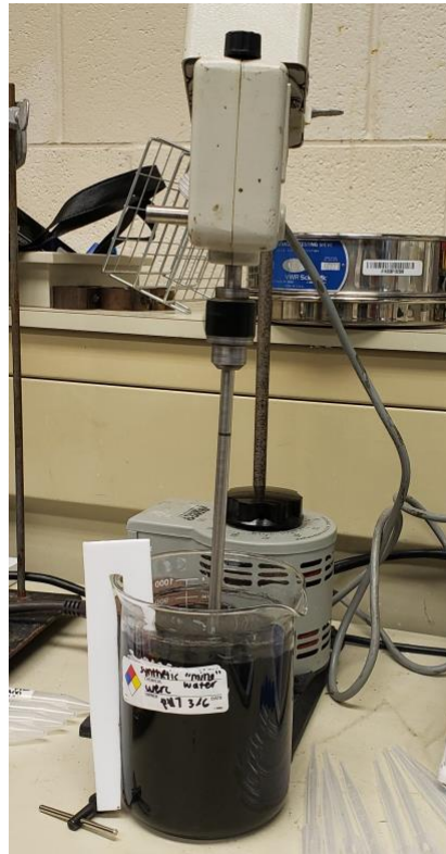
Figure 3: Batch Testing Apparatus, Bone Char
