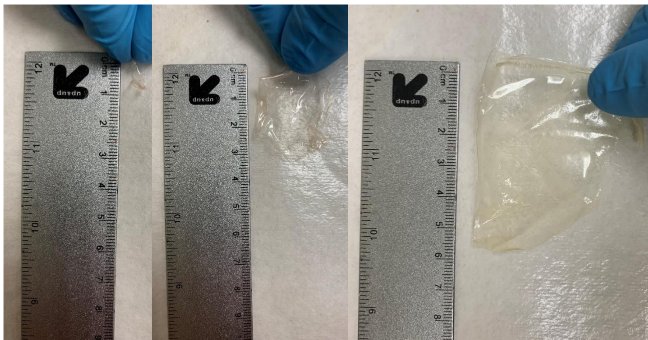
Figure 5 - Photos of a membrane from each batch of polyanilization. Smallest to largest membrane from left to right.
