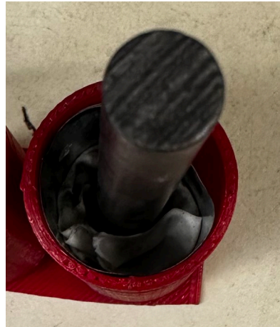
Figure 10. Image of Prototype III Zinc-Carbon Battery Instead of PVC, an ABS (Acrylonitrile Butadiene Styrene) plastic container was printed to maintain shape and sturdiness. The same construction and size zinc can were used as Prototype II, but graphite was substituted for black carbon.
