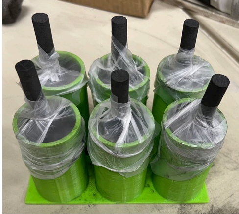
Figure 11. Image of Prototype IV Zinc-Carbon Battery A similar ABS plastic container to Prototype III was printed for Prototype IV, but the diameter was increased from two to four centimeters.
