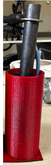
Figure 10. Image of Prototype III Zinc-Carbon Battery Instead of PVC, an ABS (Acrylonitrile Butadiene Styrene) plastic container was printed to maintain shape and sturdiness. The same construction and size zinc can were used as Prototype II, but graphite was substituted for black carbon.
