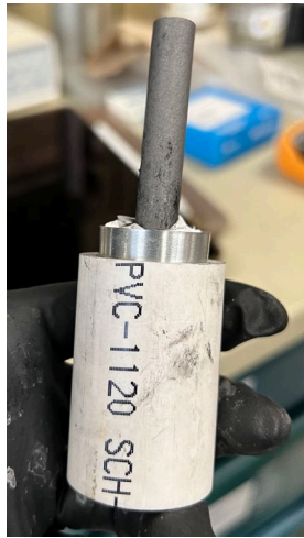
Figure 9. Image of Prototype II Zinc-Carbon Battery This prototype has a wider base, a shorter zinc can, and different cathodic material. This cathode material consisted of a carbon black base with manganese dioxide in a 3:1 ratio.
