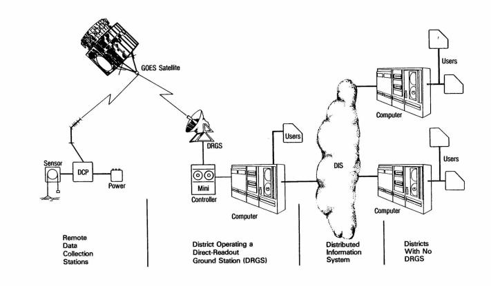
Hydrologic Data Collection Using Satellite Telemetry and a Distributed Information System
