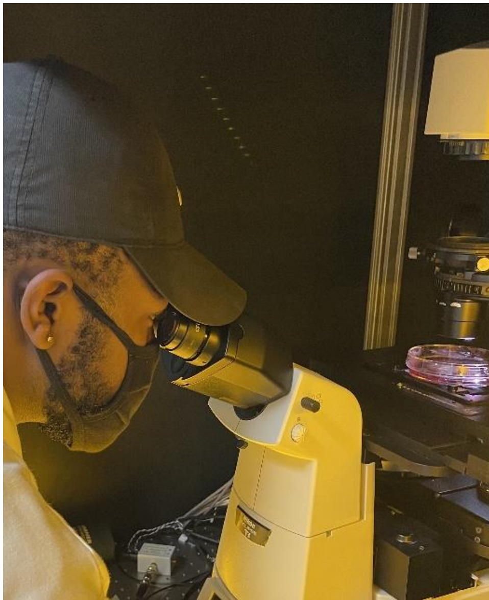
Davin Means, bringing glioblastoma cells into focus using the Bruker Ultima Investigator inverted multiphoton microscope.
