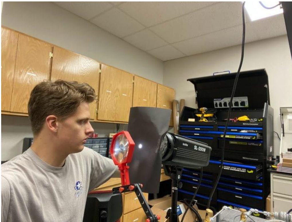
Stephen Pierson working in Dr. Han Hu’s mechanical engineering lab. Here Stephen is testing the light source collimator prototype for the solar simulator.
