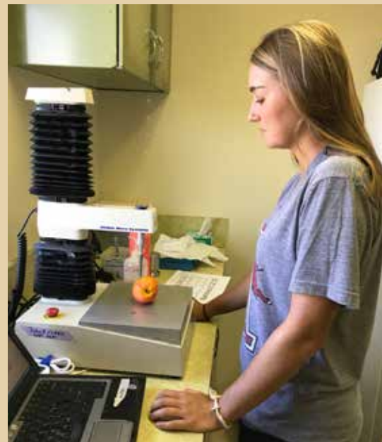
Mary Siebenmorgen measuring the firmness of a peach using a texture analyzer.
