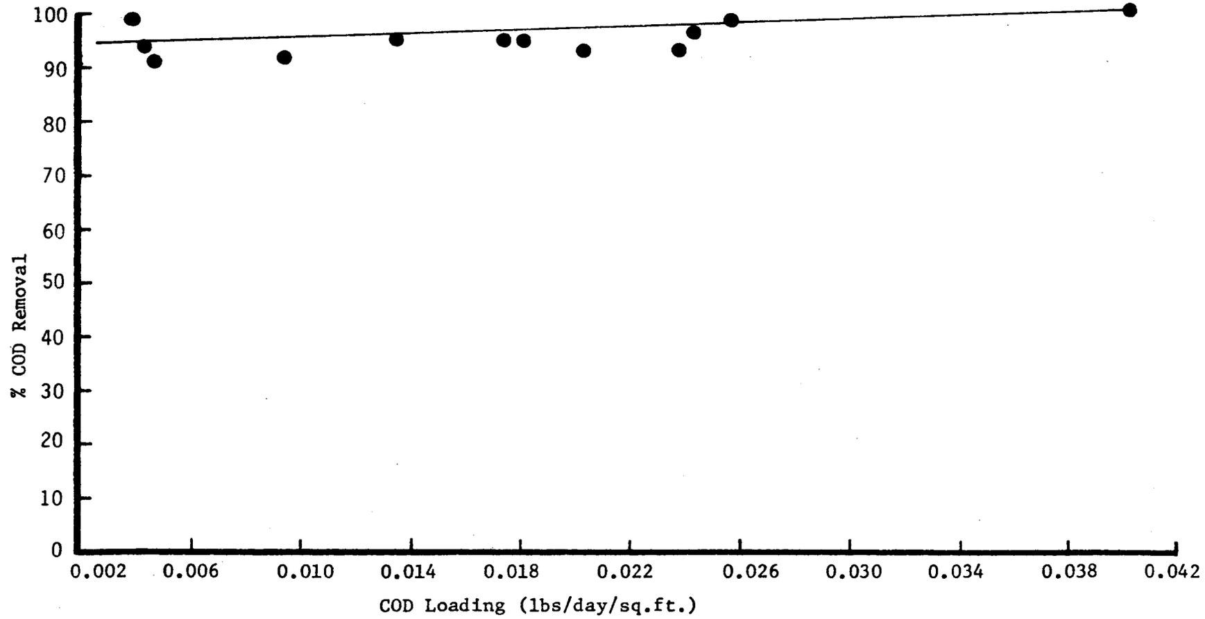
FIGURE 18 RELATIONSHIP OF COD LOADING TO COD REMOVAL FOR LYSIMETER 6 (Depth: 12 inches, Size: passed number 4 sieve)
