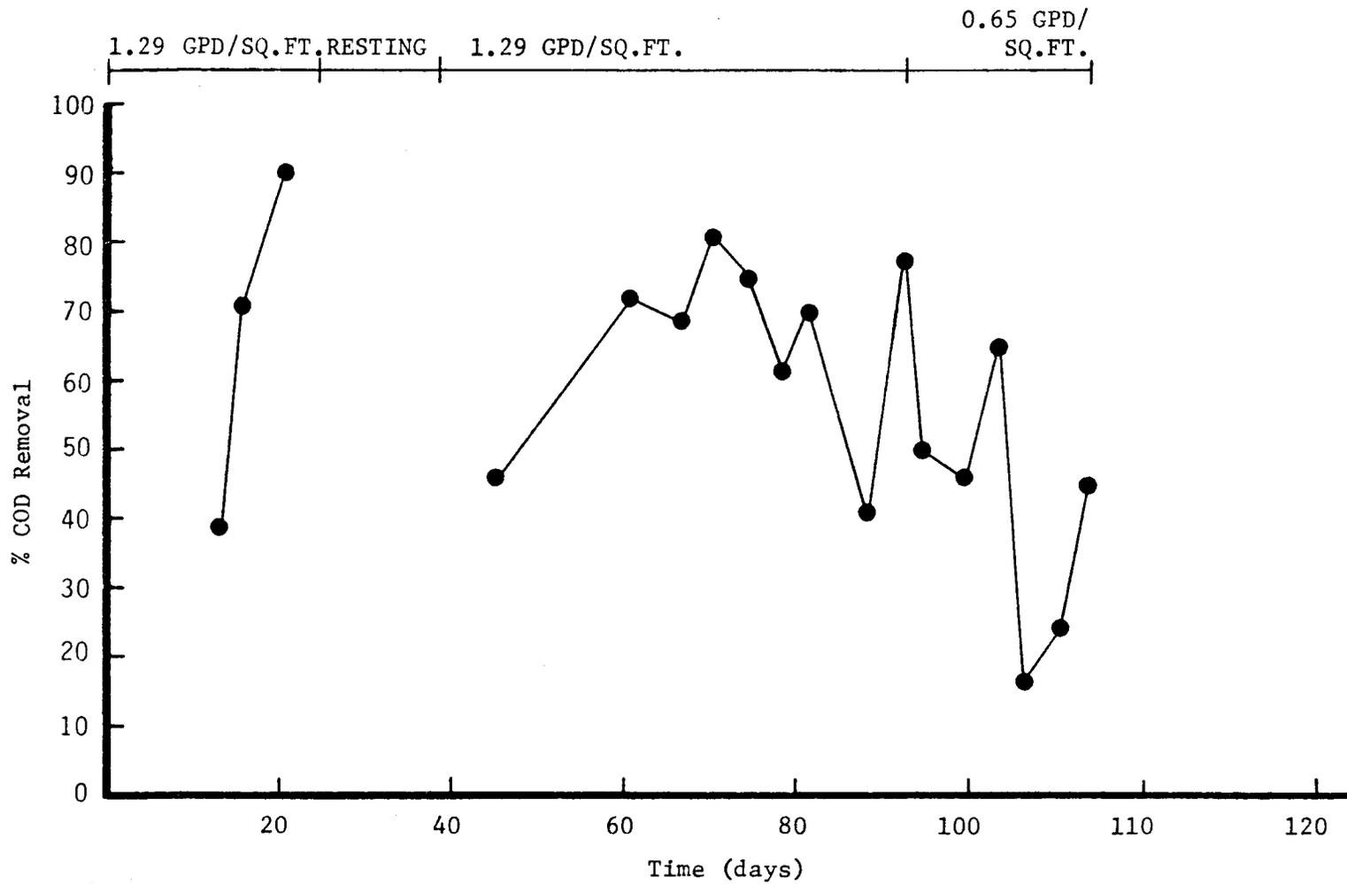
FIGURE 3 RELATIONSHIP BETWEEN TIME AND COD REMOVAL FOR LYSIMETER 13 (Depth: 6 inches, Size: passed 3/8 inch sieve)
