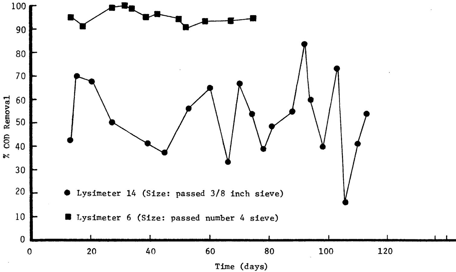
FIGURE 22 RELATIONSHIP OF COD REMOVAL TO TIME FOR LYSIMETERS OF TWELVE INCH DEPTH
