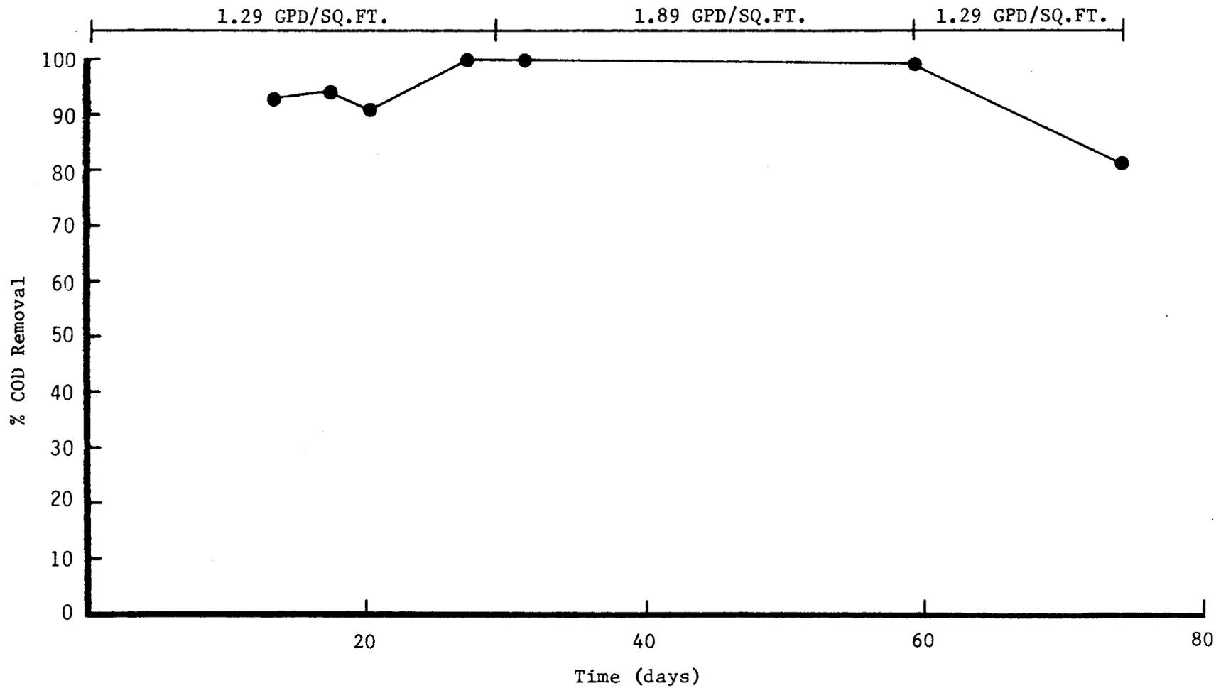
FIGURE 9 RELATIONSHIP BETWEEN TIME AND COD REMOVAL FOR LYSIMETER 8 (Depth: 18 inches, Size: passed number 4 sieve)
