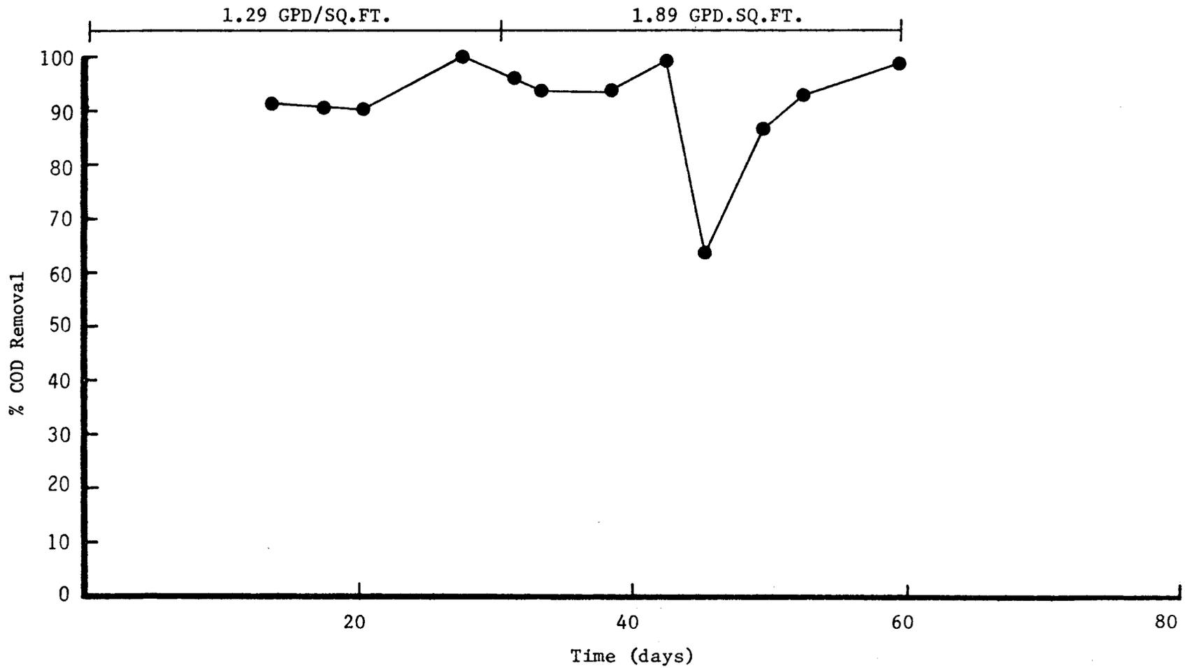
FIGURE 7 RELATIONSHIP BETWEEN TIME AND COD REMOVAL FOR LYSIMETER 5 (Depth: 6 inches, Size: passed number 4 sieve)
