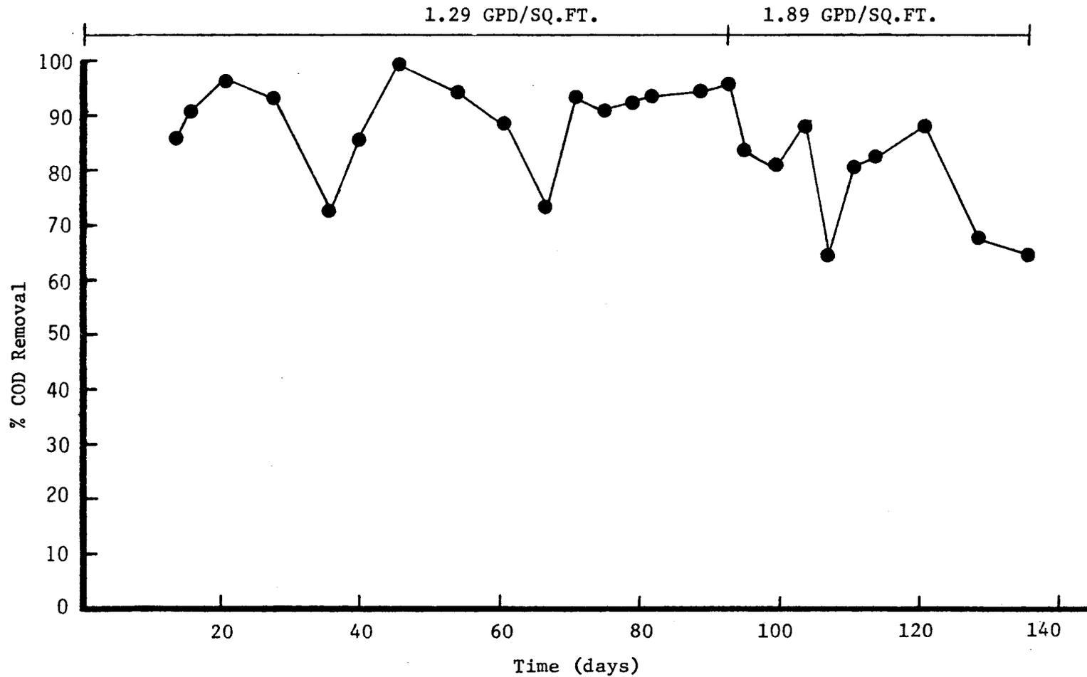
FIGURE 6 RELATIONSHIP BETWEEN TIME AND COD REMOVAL FOR LYSIMETER 15 (Depth: 24 inches, Size: passed 3/8 inch sieve)
