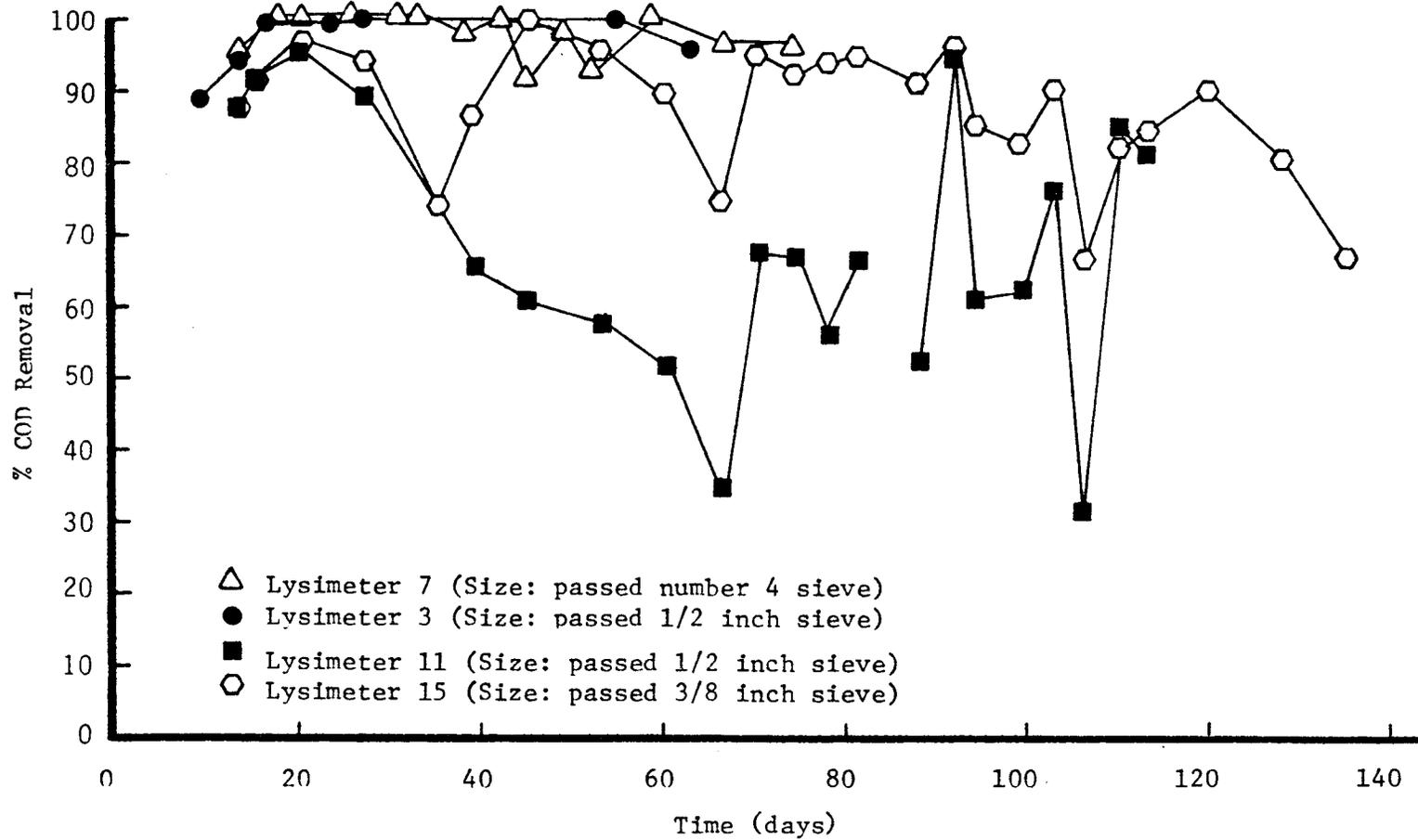
FIGURE 24 RELATIONSHIP OF COD REMOVAL TO TIME FOR LYSIMETER OF TWENTY-FOUR INCH DEPTH
