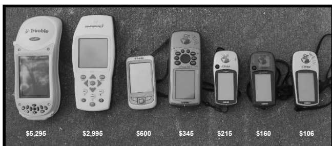
Figure 1. The seven GPS receivers tested in this study were Trimble GeoXH, Trimble GeoExplorer3, Trimble Juno, Garmin GPSMAP 76CS, Garmin eTrex Vista, Garmin eTrex Legend, Garmin eTrex (left to right with their cost shown below).
