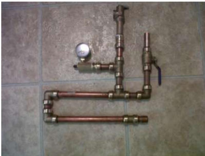
**Figure 1. Device designed to test the tendencies of CNTs during evacuation of refrigerant.**
