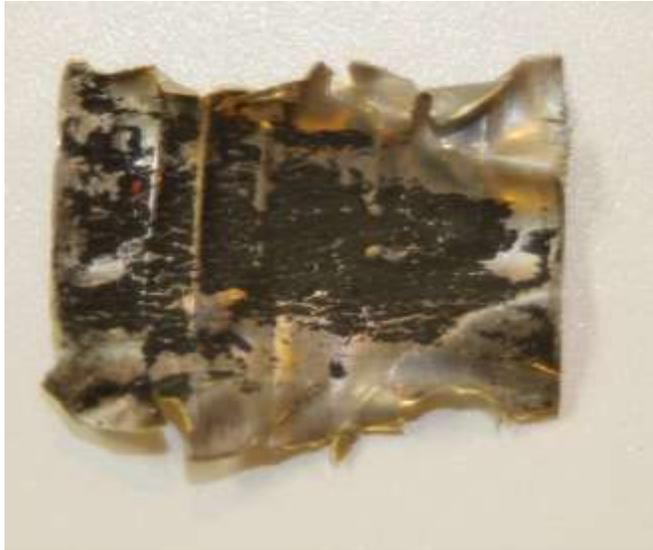
**Figure 10. Image of CNT buildup on the one inch transition piece from copper tube pre-condenser manifold to aluminum tube condenser.**
