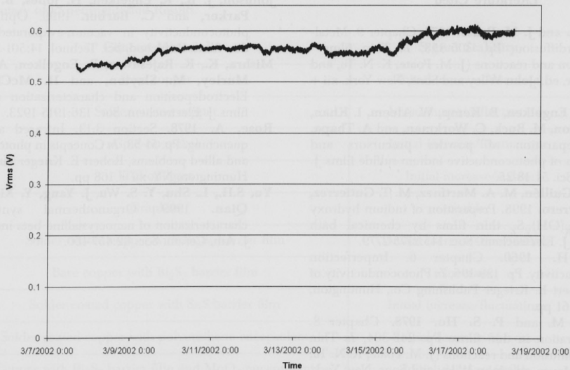
Fig. 14. Stability of photovoltage for \text{In}_2\text{S}_3 on graphite contacts over time.
