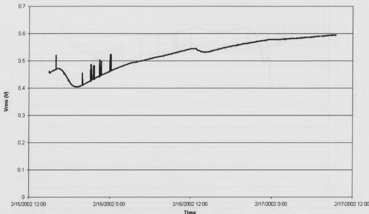
Fig. 15. Stability of photovoltage over time for \text{In}_2\text{S}_3 with polyurethane encapsulation.
