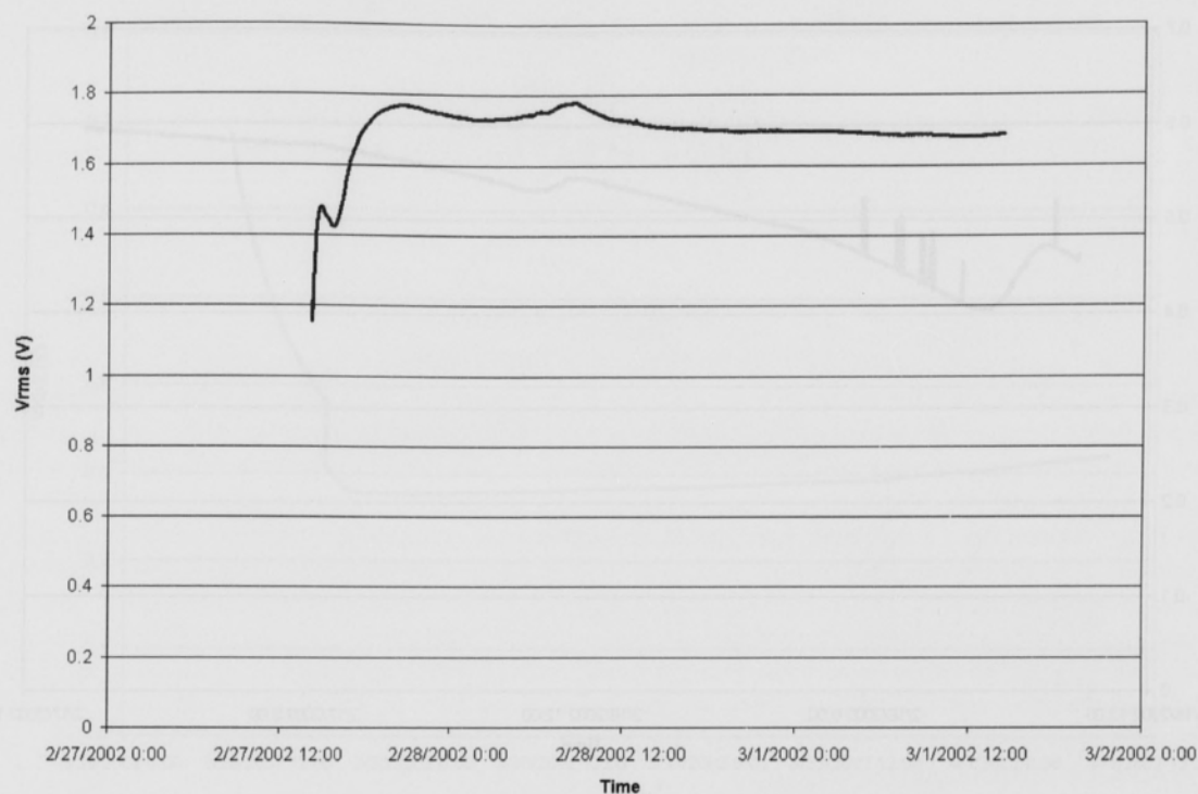
Fig. 13. Stability of photovoltage for \text{In}_2\text{S}_3 on ITO-on-glass contacts over time.
