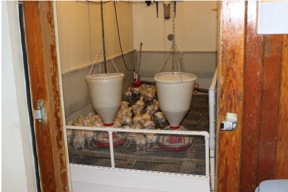
Figure 1. Pens constructed with flat wire flooring and placed within ten environmental chambers (dimensions: 3.7 m long x 2.5 m wide x 2.5 m high) at the University of Arkansas Poultry Research Farm. Feeders were placed at the front of the pen and a nipple watering system was placed at the back of the pen forcing the birds to travel the length of the pen to eat and drink. This experimental model reproducibly triggers significant levels of lameness attributable to BCO.
