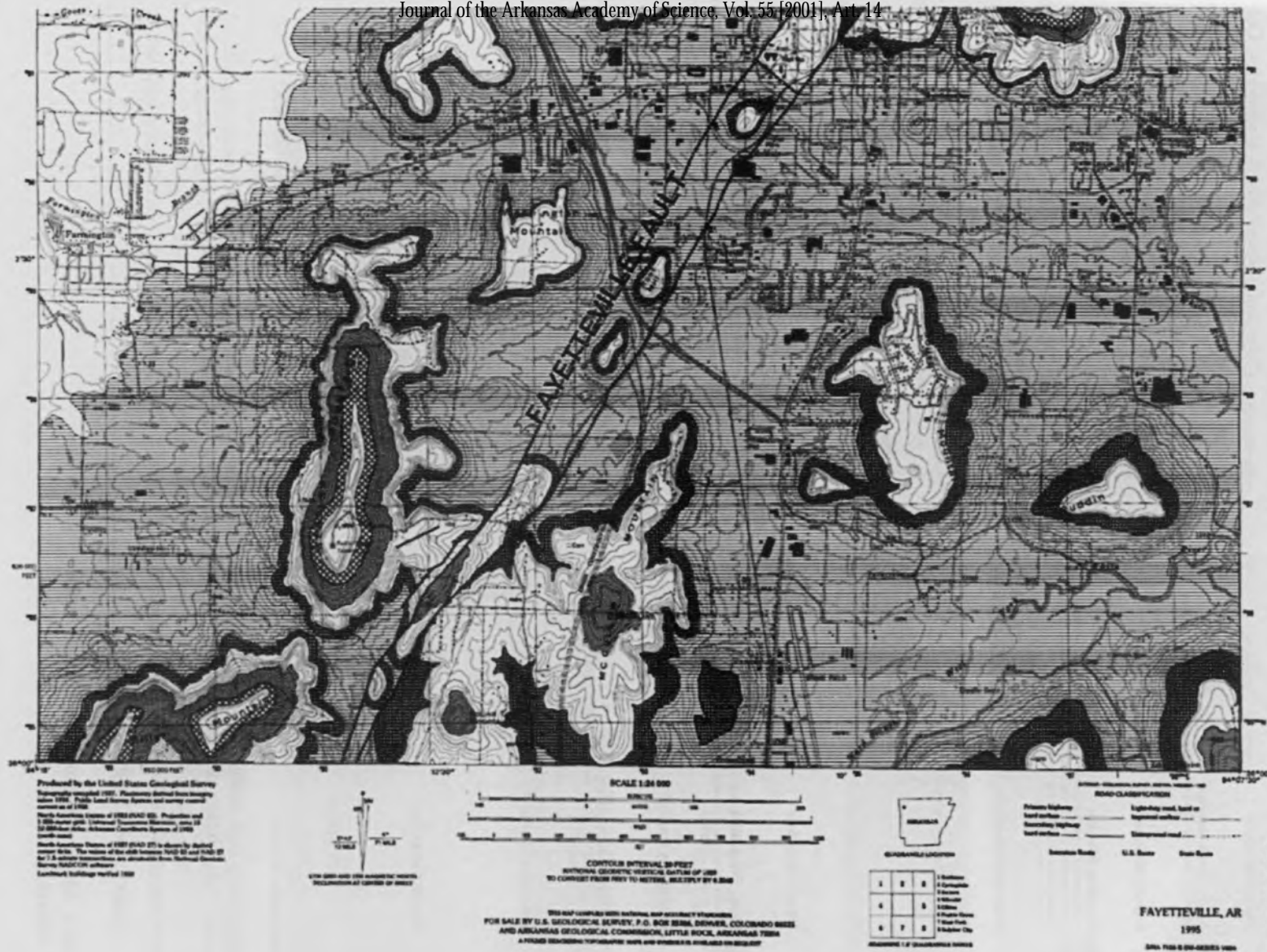
Fig. 3. Map of southern half of Fayetteville 7.5-Minute Quadrangle, Arkansas showing outcrop extents of shale strata containing swelling clays and known to weather to expansive soils.
