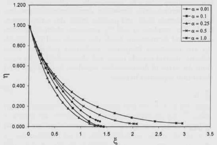
Fig. 2. Electric field,  $\eta$ , as a function of position inside the sheath,  $\xi$ , for five values of  $\alpha$ .  $\alpha = 0.01, 0.1, 0.25, 0.5$ , and  $1$ .  $\alpha$  represents wave speed.
