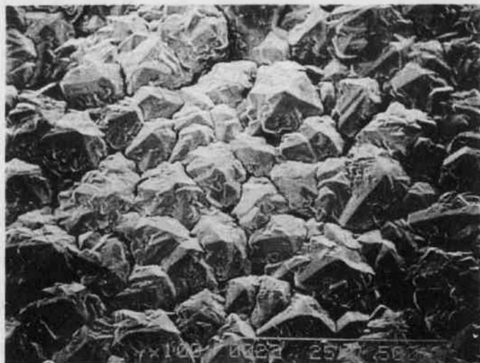
Fig. 3. Scanning electron micrograph of a diamond substrate etched at a low pressure (150 mTorr) in the chamber (showing preferential etching along grain boundaries).
