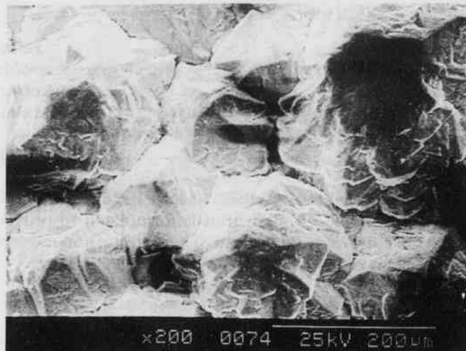
Fig. 7. (a). Scanning electron micrograph of a CAMP-polished diamond substrate with reactive ion etching.
