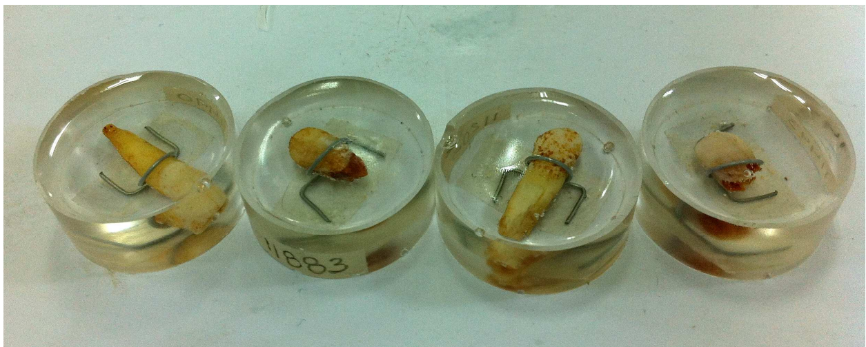
Figure 4.3: Tooth samples embedded in cured epoxy resin with round shape. (Photograph by Teresa Wilson)
