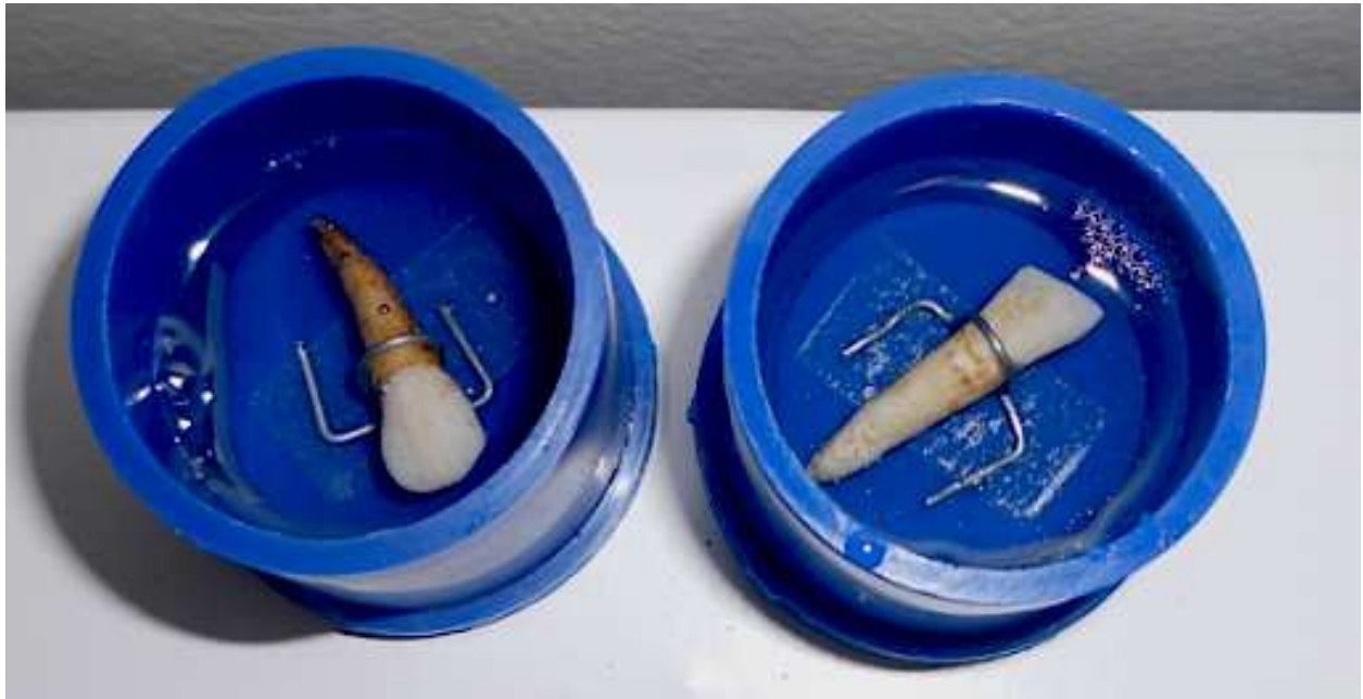
Figure 4.2: Teeth secured inside Leco cups and embedded in Araldite epoxy resin. (Photograph by Teresa Wilson)
