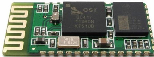
Figure 5.1 – Bluetooth HC-05 Module
