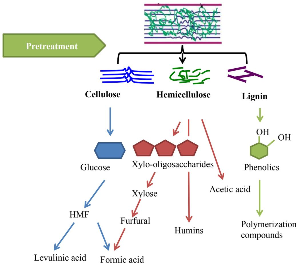
**Figure 1.** A schematic representation of degradation products formed during typical physico-chemical deconstruction of lignocellulosic biomass.<sup>19,52,53</sup>
