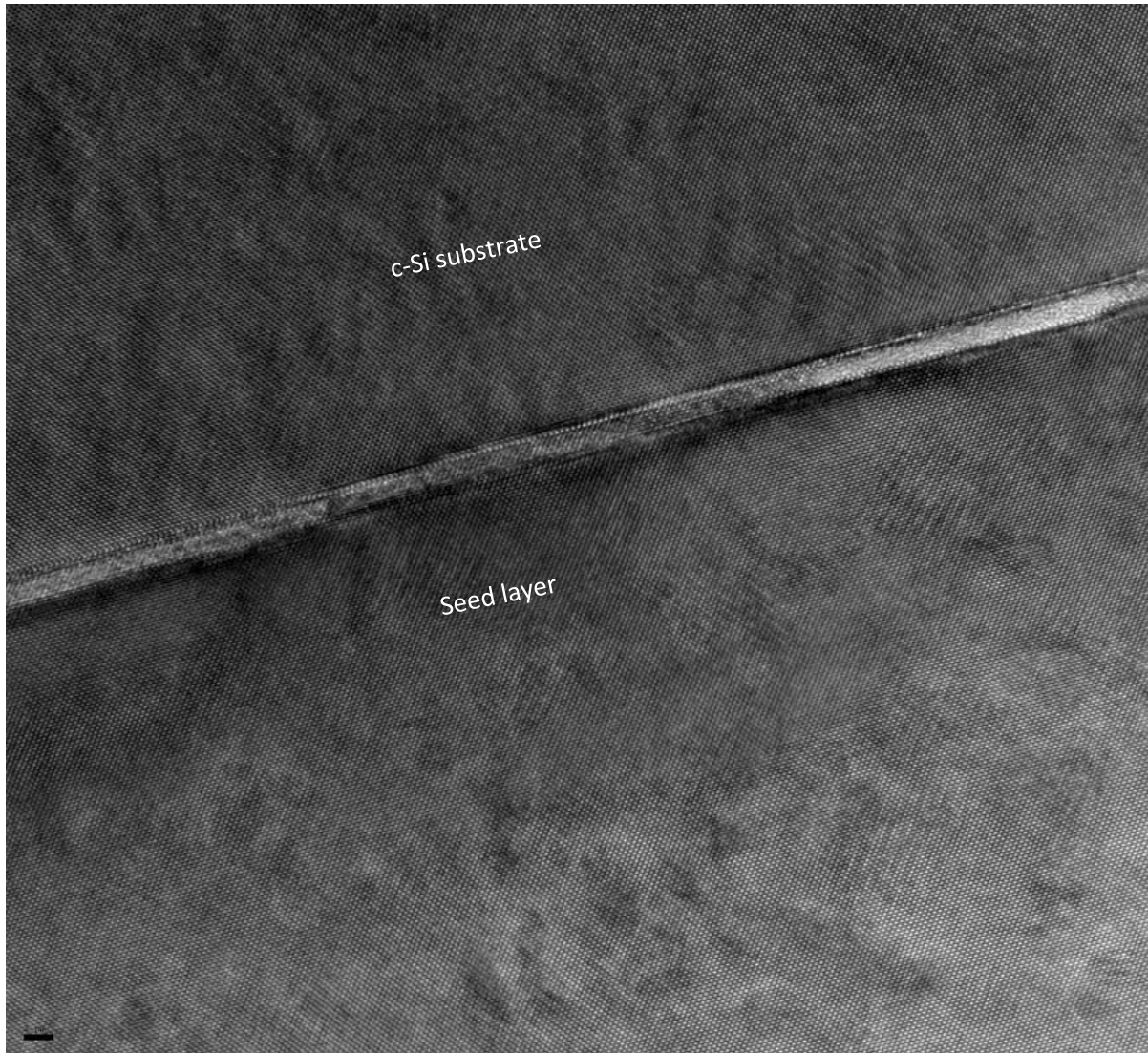
Figure 51. A cross-sectional TEM image that shows the single layer of Si that were growing using AIC.
