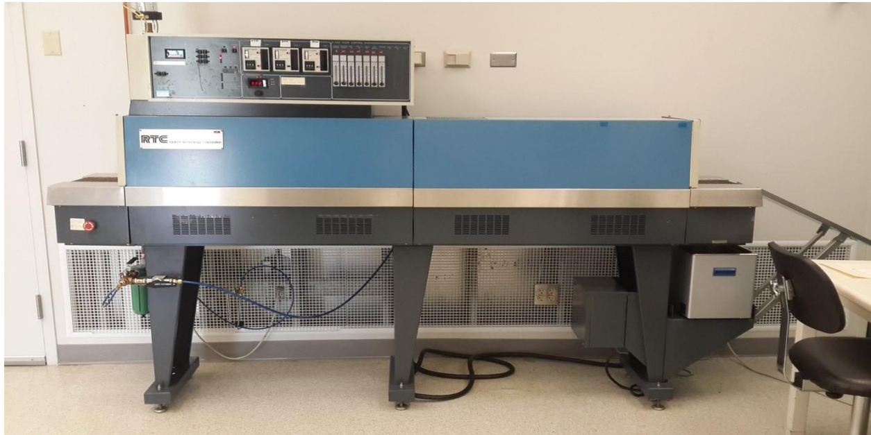
Figure 11. The IR-Belt furnace at HiDEC (picture taken by the author).
