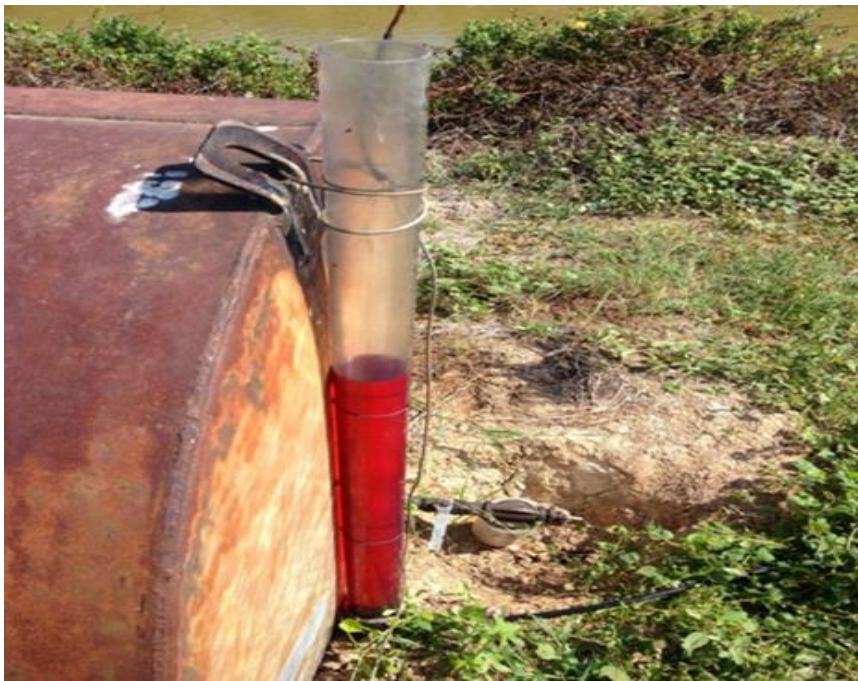
Figure 3. Graduated Cylinder Method of Diesel Fuel Flow Measurement.
