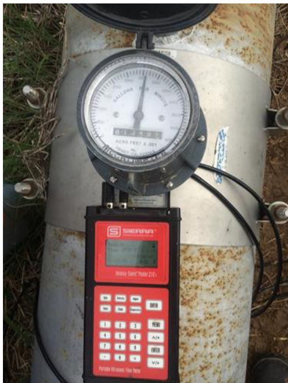
Figure 8. Cross-Checking Flow Values of a McCrometer Saddle Propeller Flowmeter and a Sierra 210i Ultrasonic Flowmeter.
