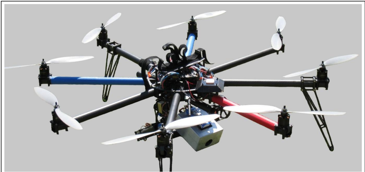
Figure 23: The Cinestar 8 with FLIR in aluminum case mounted on the gimbal (Image: Autumn Cool).
