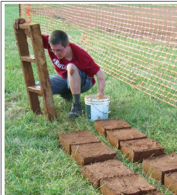
Figure 5: Mudbricks dry in the sun while a student prepares the mold for a new batch (Image: Autumn Cool).
