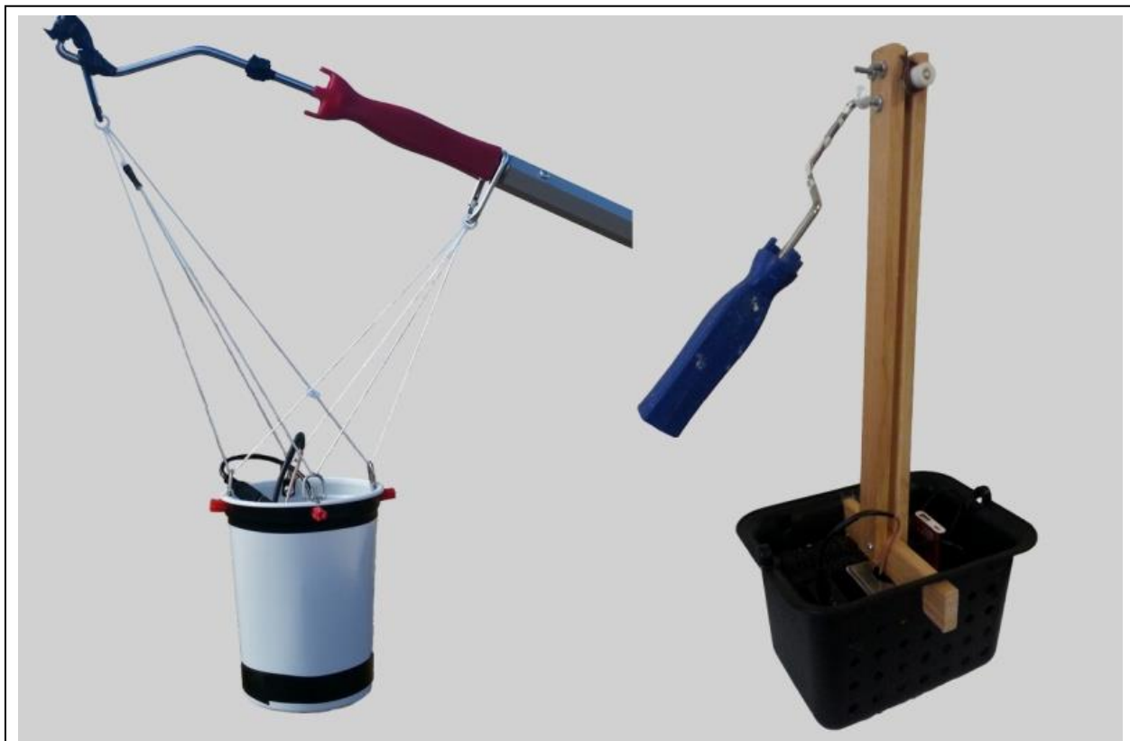
Figure 7: The string picavet (left) and the hinged suspension system (right) (Image: Autumn Cool).
