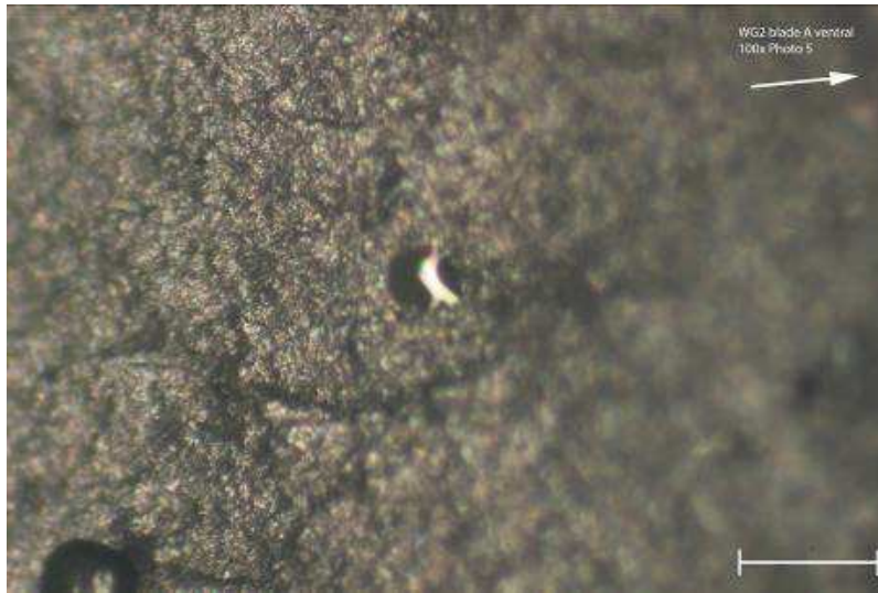
Figure 16: WG2 blade A ventral side at 100x, location 5. An oil spot is visible in the center of the frame. Scale bar is 100 microns long.
