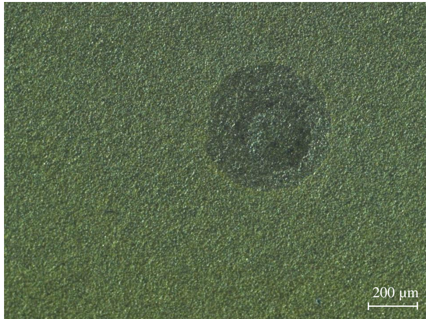
Fig. 5.16. A pristine via covered with large pin pull test pad.
