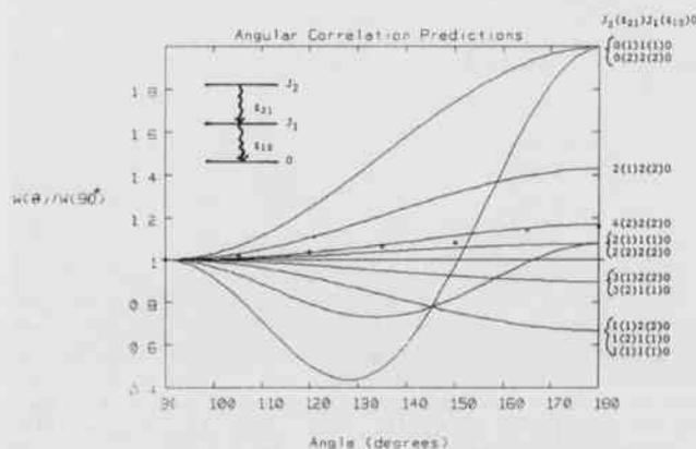
Figure 2. Predictions for eleven different combinations of excited state spins and de-excitation gamma ray multiplicities, the latter given in parenthesis. Data for  $^{60}\text{Ni}$  are the small boxes.
