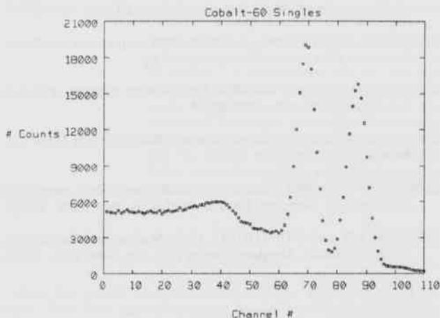
Figure 4. Gamma ray singles from either small NaI detector.
