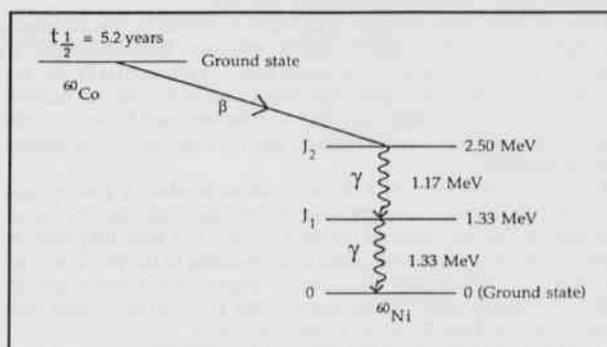
Figure 1. Decay scheme for radioactive  $^{60}\text{Co}$ .
