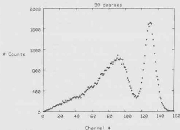
Figure 5. Coincidence gamma-gamma sum spectrum for  $^{60}\text{Ni}$ .
