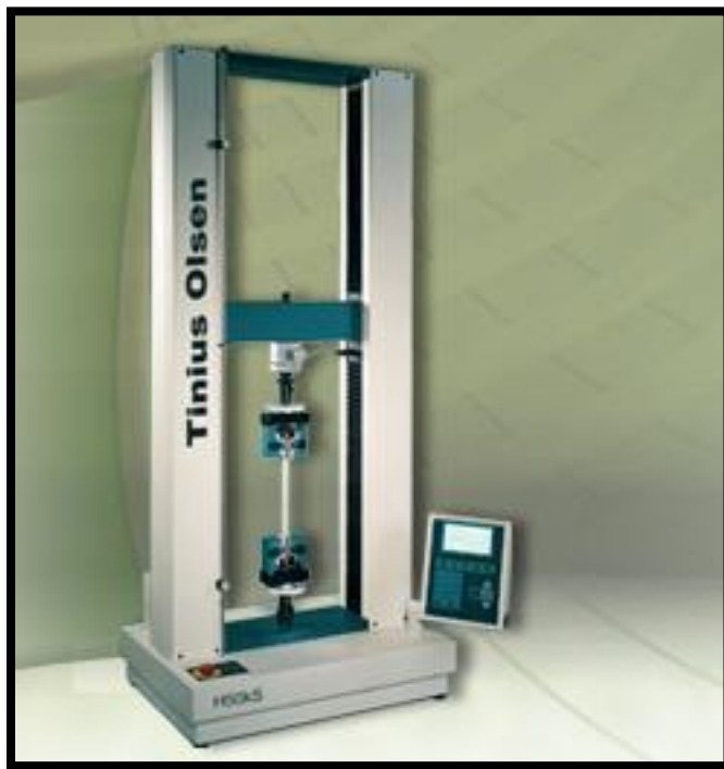
Figure 18. Tinius Olsen H50KS tensile tester. [www.tiniusolsen.com]
