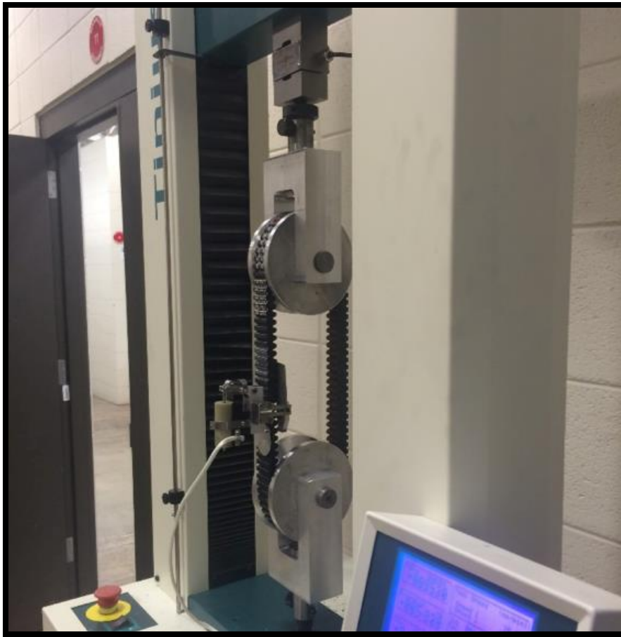
Figure 20. Tensile test-fixture and setup.
