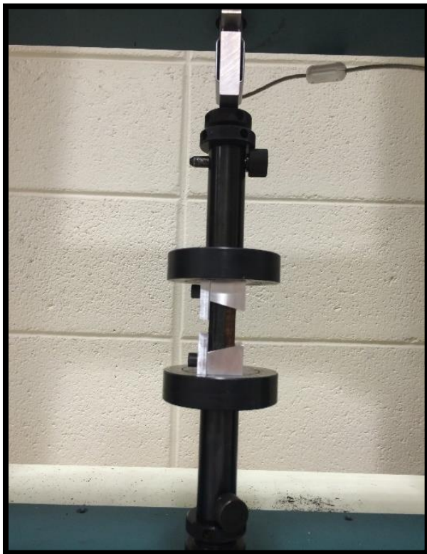
Figure 32. Test setup for v-block adaptor compression test.
