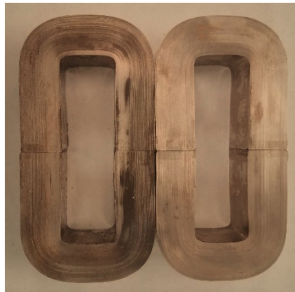
Fig. 4.3. Two sets of C-cores AMCC-50 in a shell-type configuration
