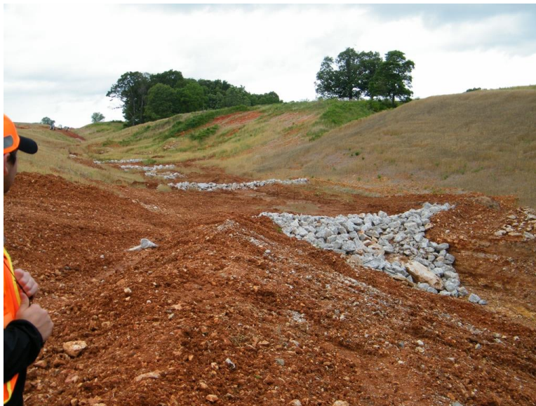
Figure 3.2: Photograph of the site chosen for the first field test. One inflow stream was from the left side of the photo, which enters the small and shallow basin. A second inflow stream is pictured in the background, which included a series of small basins with intermittent rock checks. Photo taken by Bryan Signorelli (AHTD) on June 18, 2015.
