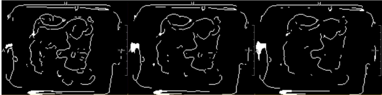
Figure 4.22: Results of the Canny edge detector on the same dataset using sigma value equal to 3, 4, and 5, respectively.
