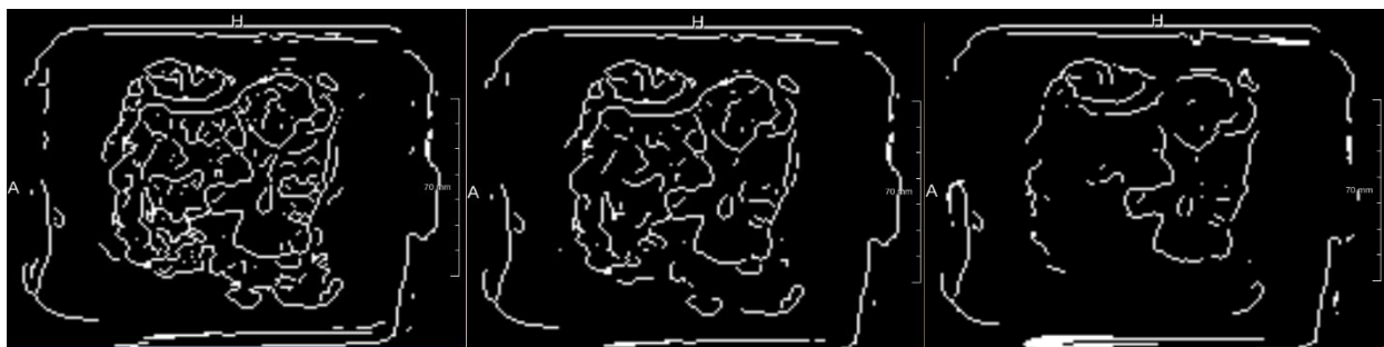
Figure 4.21: Results of the Canny edge detector on one of our dataset using low threshold value 0.02, 0.03, and 0.04, and high threshold value 0.06, 0.09, and 0.12, respectively.
