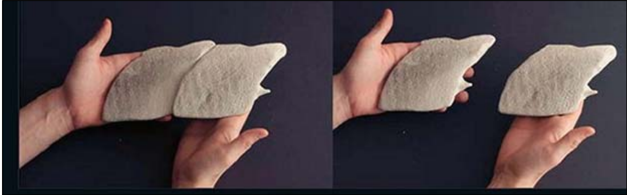
Figure 2.6 3-D printed prototype demonstrating peg-and-socket joint connecting the adjacent overlapping birchir ganoid scales [Images courtesy of the U.S. Army's Institute for Soldier Nanotechnology located at Massachusetts Institute of Technology].
