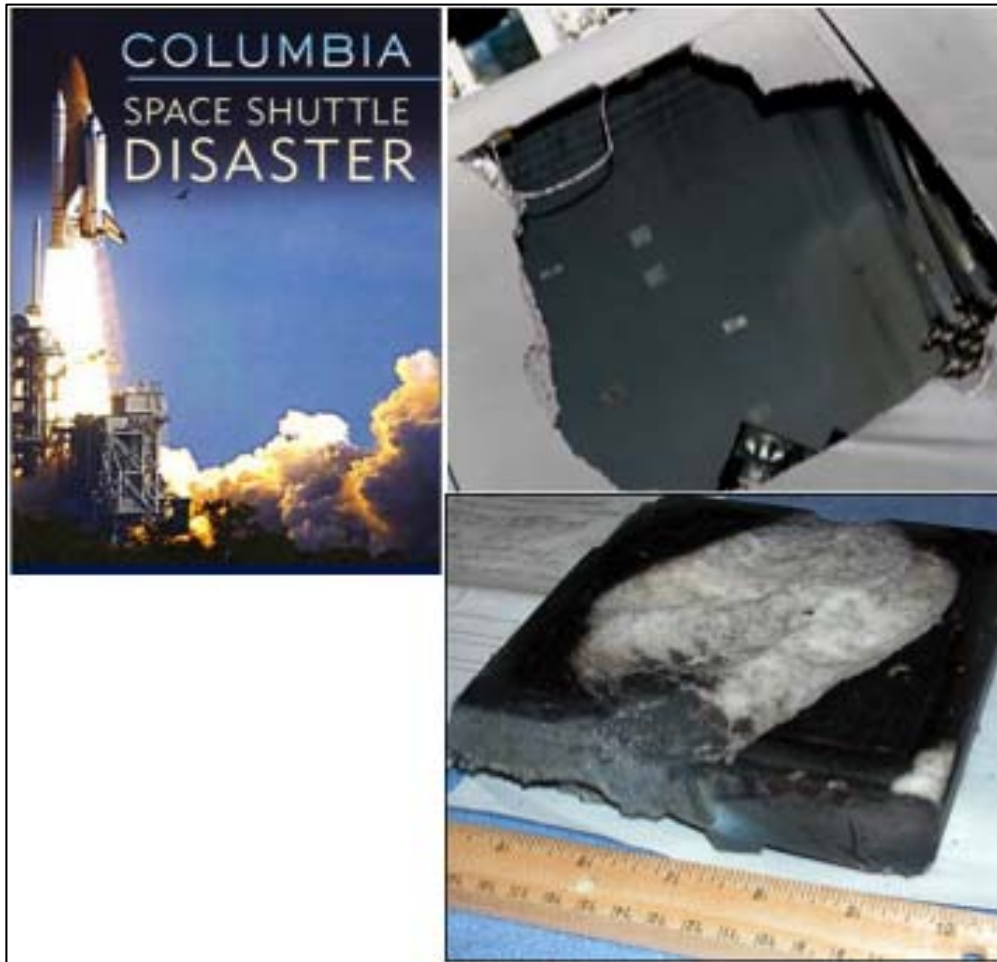
Figure 1.2 Composites fail by delamination when impacted, foam-tile delamination led to Columbia space shuttle disaster (Columbia Accident Investigation Board, 2003).
