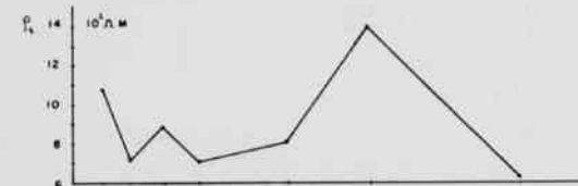
Figure 3B. Apparent resistivity of a Schlumberger profile with an electrode separation of 80 m.
