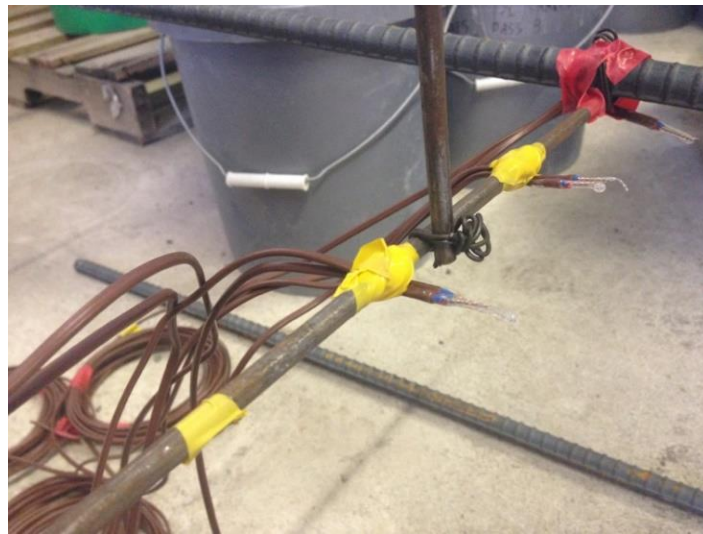
Figure 3.3 – Internal Type II thermocouples
