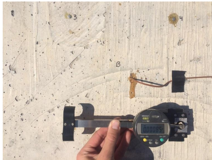
Figure 3.4 – Expansion/strain measurement with DEMEC gauge
