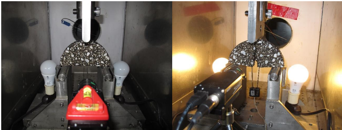
Figure 4.3 SC(B) Test Configuration, Before(left) and After(right) Test
