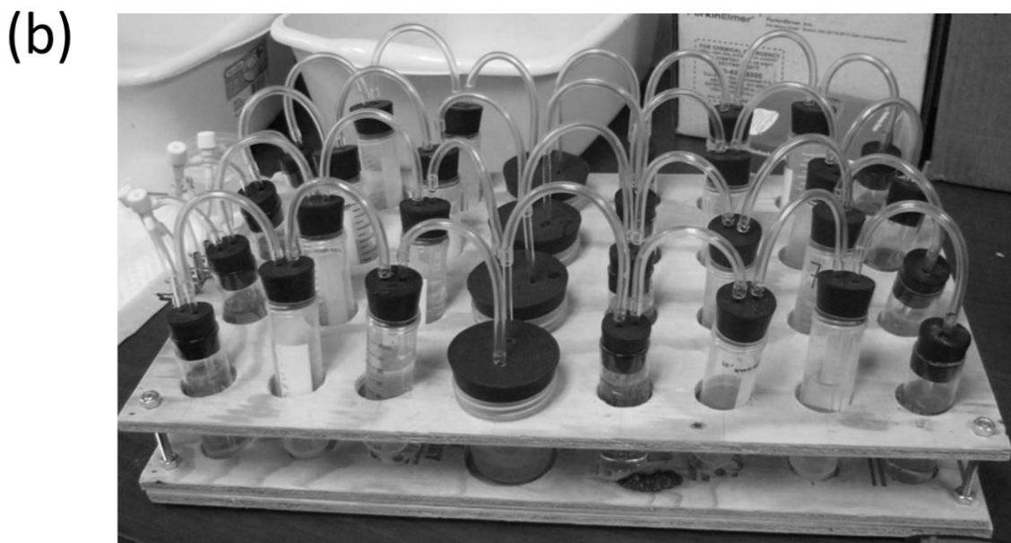
Figure S1. (a) Design of radiation chambers used in caddisfly radiolabel experiments. Potassium hydroxide (KOH) served as a trap for CO 2 entering and leaving the system to prevent release of 14 C-CO 2 , whereas air and water (H 2 O) chambers served as safety traps and buffer chambers respectively to prevent transmittance of KOH to the insect chamber (fourth from left). Each series of tubes was replicated to permit radiolabeling of 20 individuals from each genus. (b) Final constructed version of chambers (1 rack containing tubes for 4 total labeling chambers) used in experiments.
