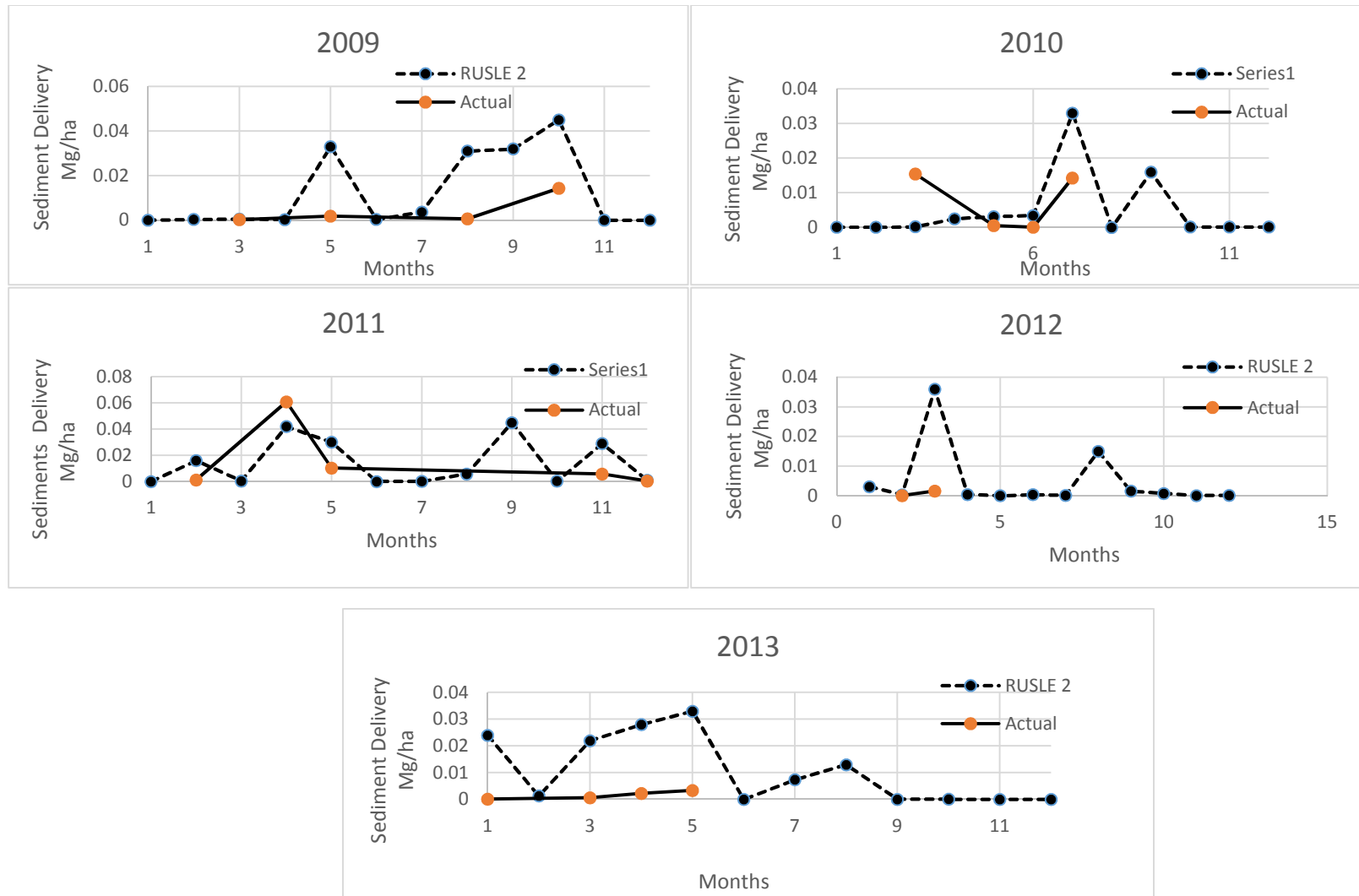
Figure 4.4.2.1.4 Comparison of the temporal variation of RUSLE 2 and Measured Sediment Delivery for Site HE4
