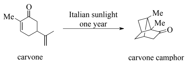
Figure 3.1. Ciamician’s Conversion of Carvone to Carvone Camphor using Sunlight
