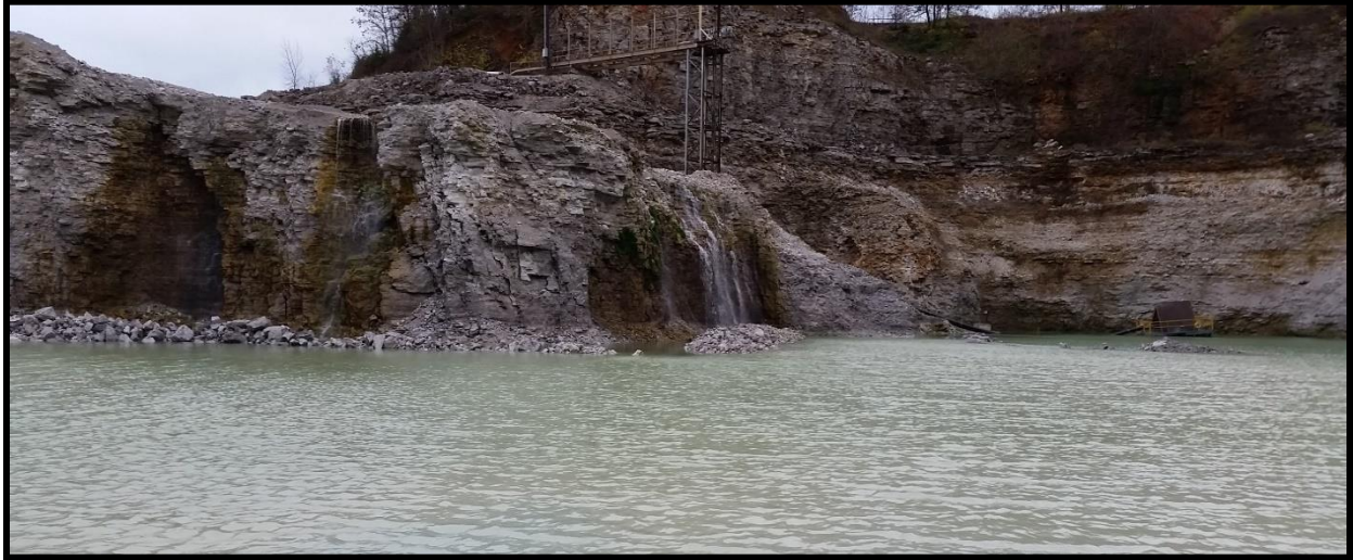
Figure 7. A picture of the Sharp's Quarry sump where water samples were collected during stormflow. Water can be seen entering the sump from bedding planes in the quarry walls.
