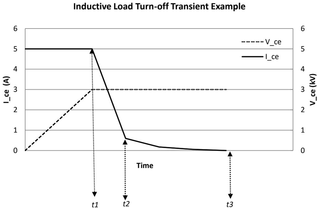
Figure 2.3 Example of an inductive load turn-off response.
