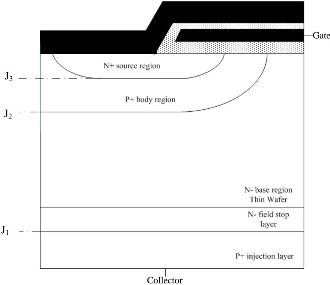
Figure 1.1 Cross section of an n-channel IGBT.
