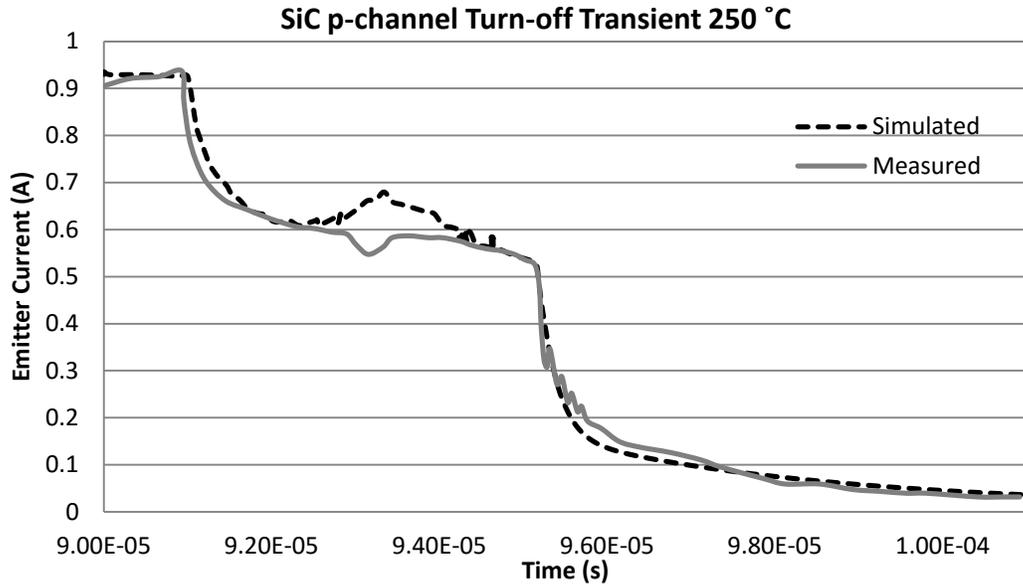
Figure 6.20 SiC p-channel turn-off current characteristics at 250 °C.
