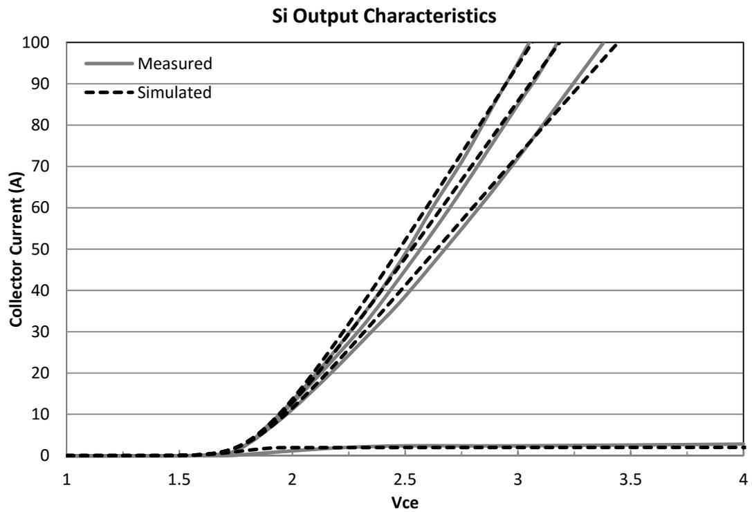
Figure 6.2 Si IGBT Output Characteristics at 25 °C.
