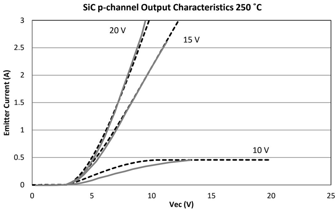
Figure 6.16 SiC p-channel output characteristics at 250 °C.
