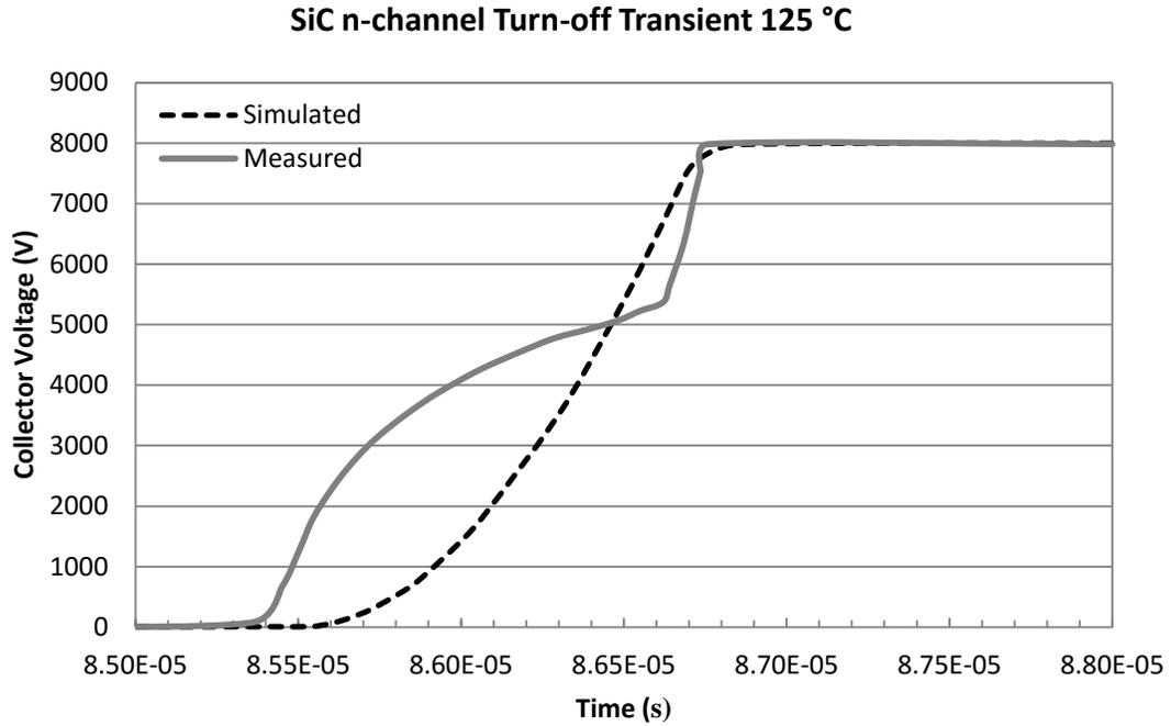
Figure 6.14 SiC n-channel turn-off voltage characteristics at 125 °C.
