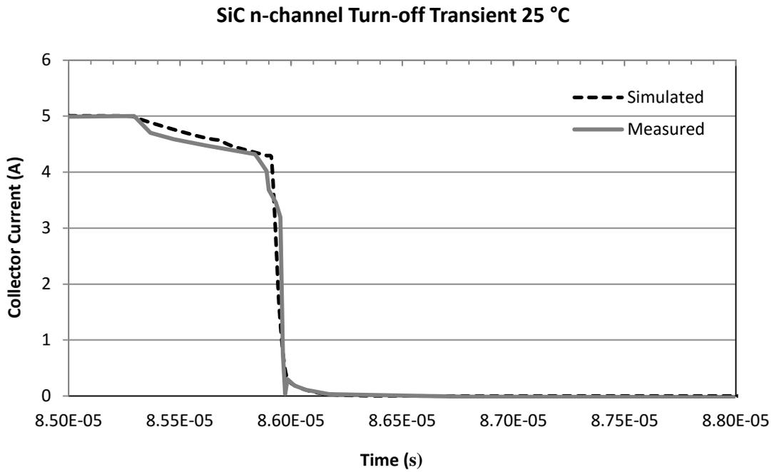
Figure 6.13 SiC n-channel turn-off current characteristics at 25 °C.
