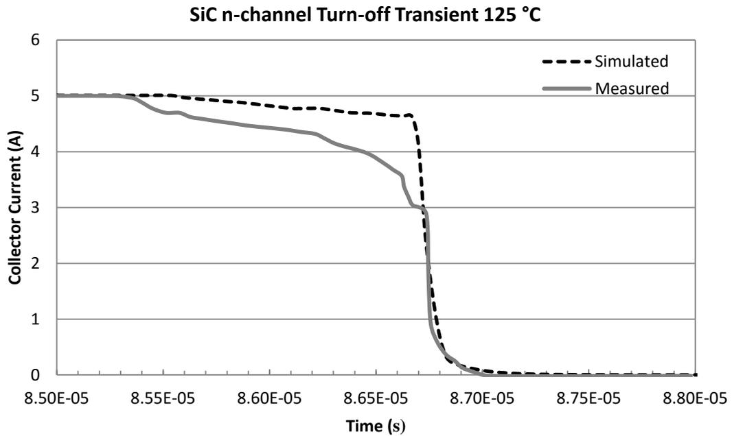
Figure 6.15 SiC n-channel turn-off current characteristics at 125 °C.
