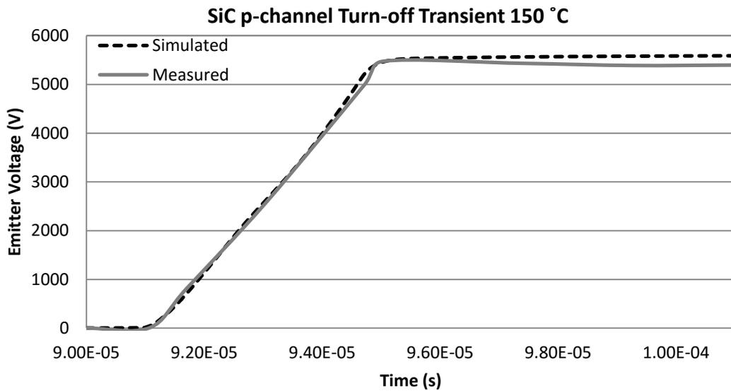
Figure 6.19 SiC p-channel turn-off voltage characteristics at 150 °C.
