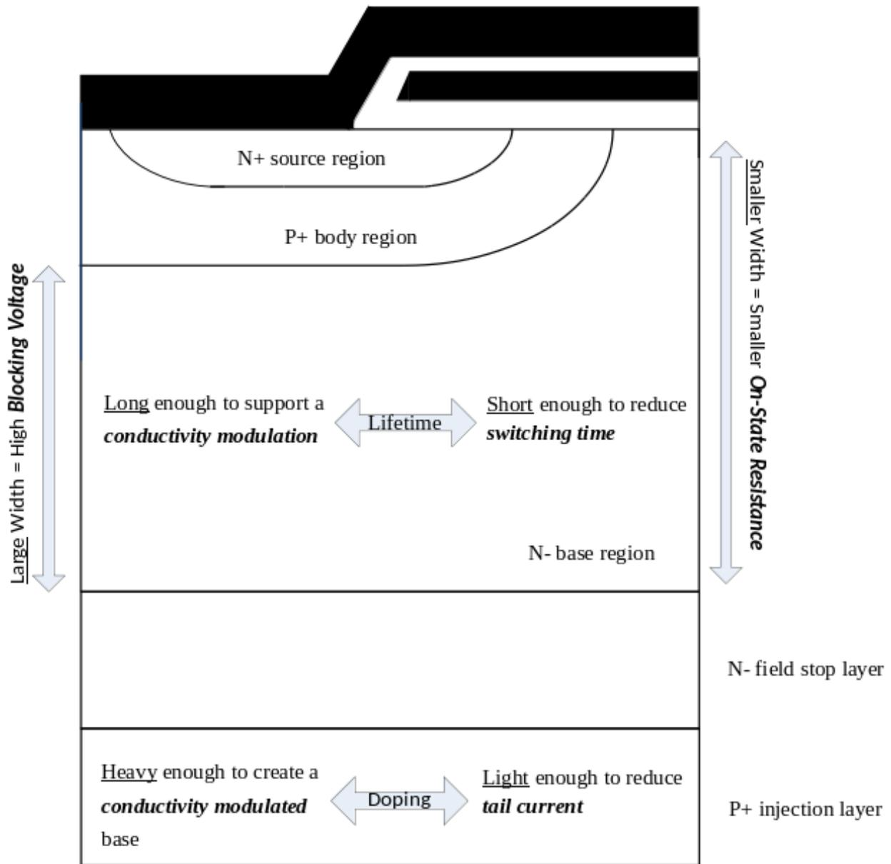
Figure 2.6 Trade-offs of designing an IGBT by layer.
