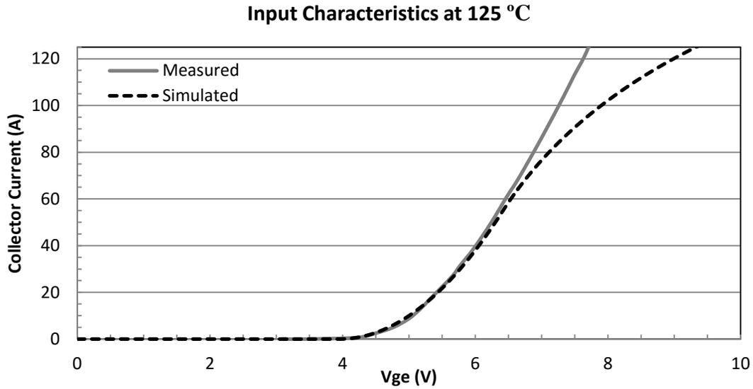
Figure 6.9 Si IGBT input characteristics at 125 °C.
