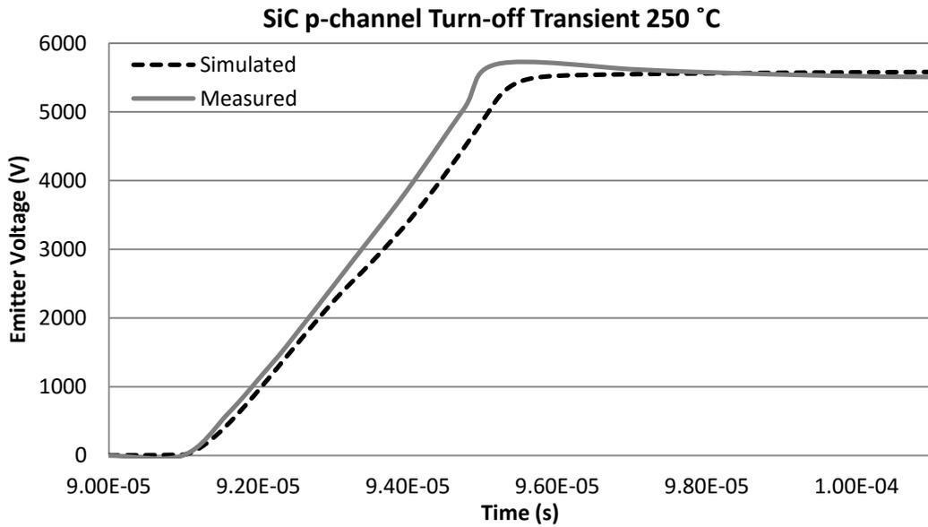
Figure 6.21 SiC p-channel turn-off voltage characteristics at 250 °C.
