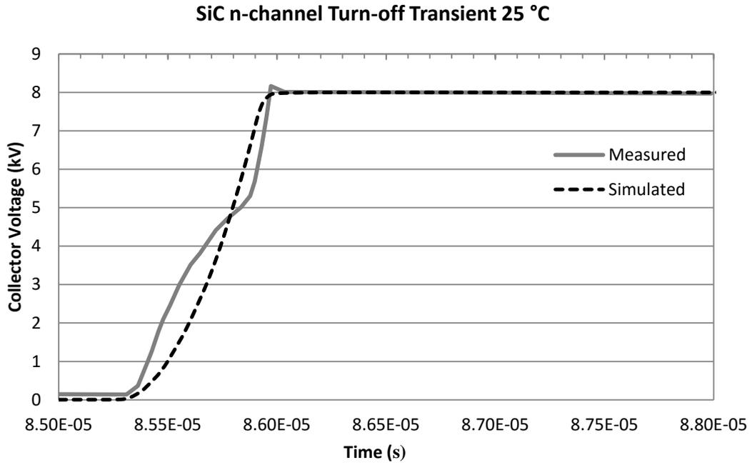
Figure 6.12 SiC n-channel turn-off voltage characteristics at 25 °C.
