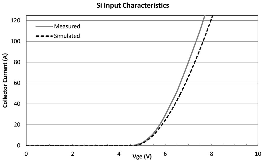
Figure 6.3 Si IGBT Input Characteristics at 25 °C.
