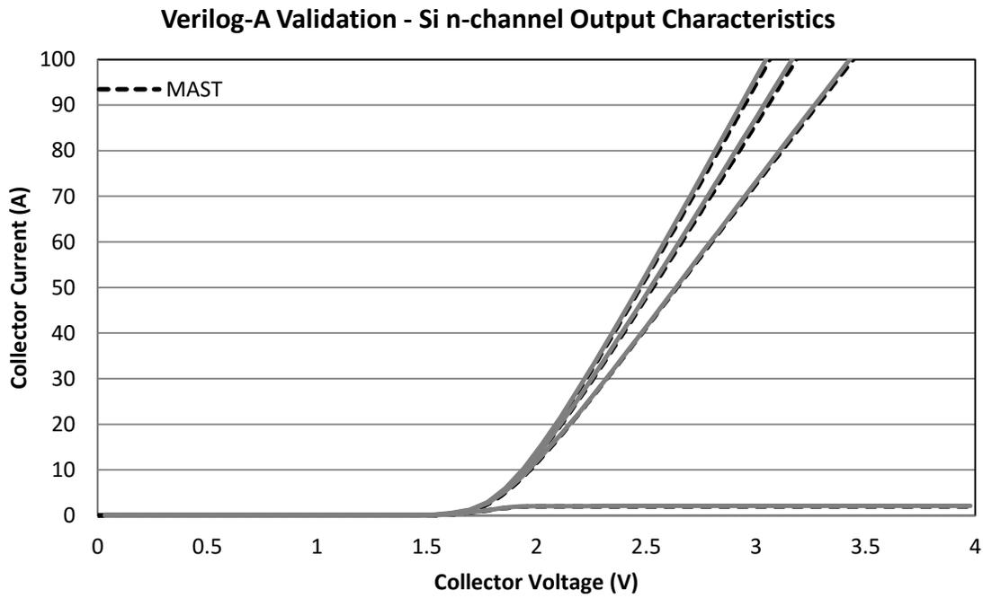
Figure 6.23 Si output characteristics Verilog-A validation.
