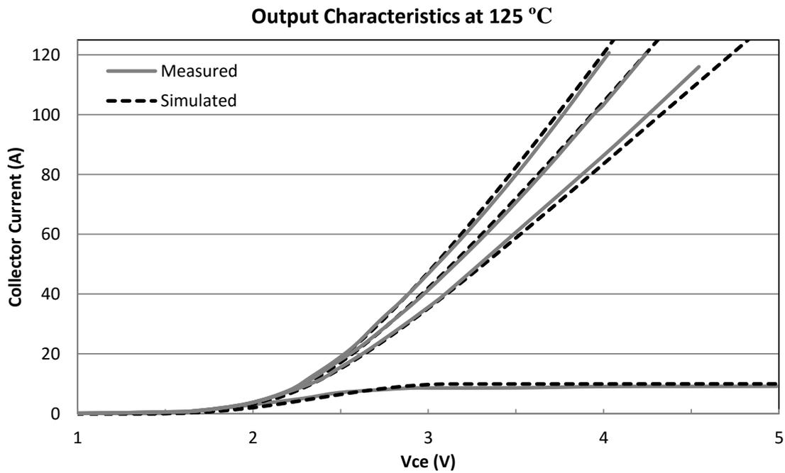
Figure 6.8 Si IGBT output characteristics at 125 °C.
