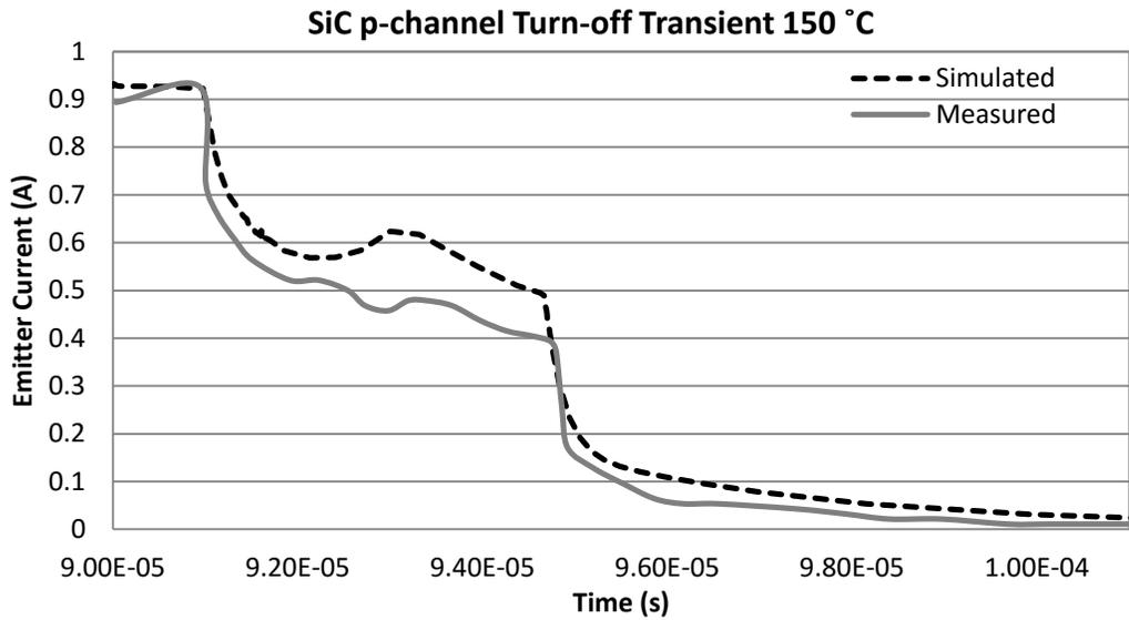
Figure 6.18 SiC p-channel turn-off current characteristics at 150 °C.
