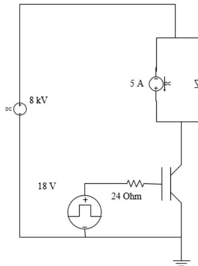
Figure 6.11 SiC n-channel IGBT clamped-inductive load testbench.
