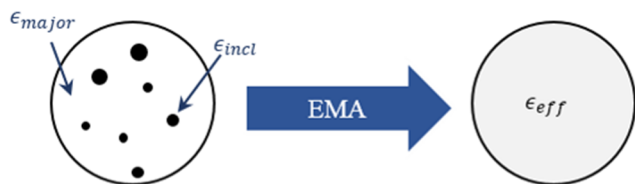
Figure 1: The diagram illustrates how effective medium approximations (EMAs) simplify the treatment of a particle containing randomly placed inclusions. By inputting the permittivities of the components with their respective volume fractions, the EMA computes an effective permittivity, \epsilon_{eff} , of the homogenized particle for use in Mie scattering calculations.
