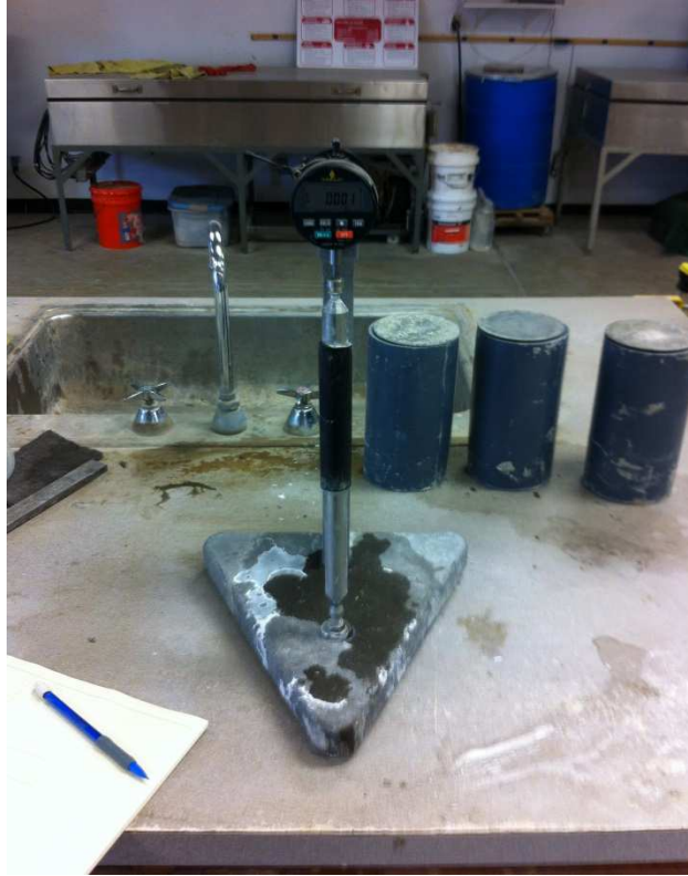
Figure 3.4. Length Change Comparator
