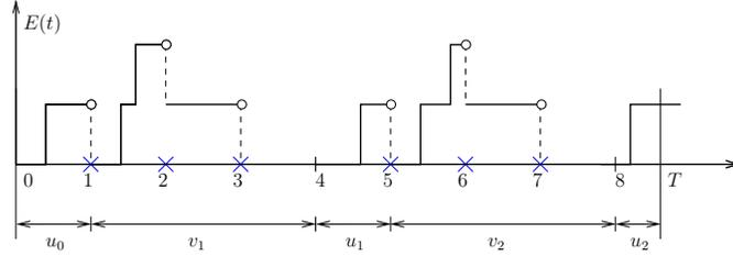
Figure 2.6: An energy level evolution sample path. Crosses represent actual sensing epochs.
