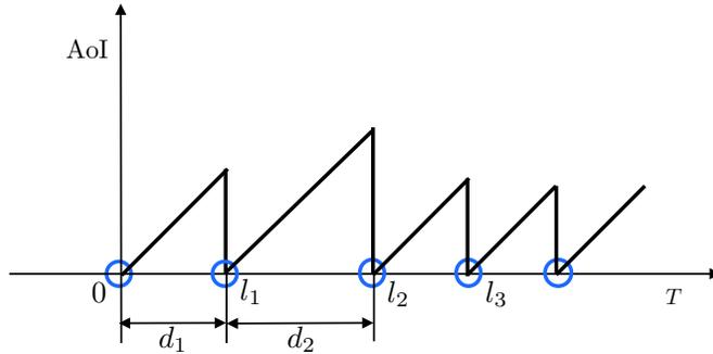
Figure 3.1: AoI as a function of  $T$ . Circles represent status update instants.
