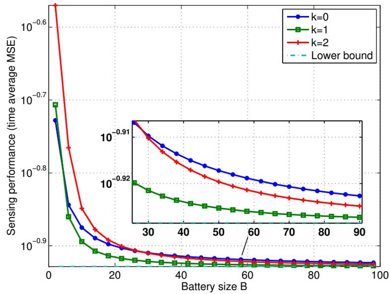
Figure 2.5: The time averaged sensing MSE.
