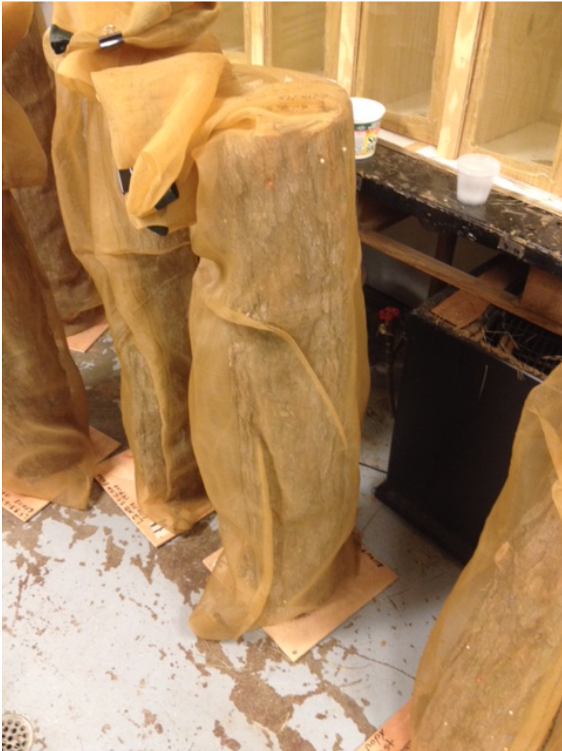
Individual experimental shortleaf pine bolts wrapped in Lumite mesh and screwed to a flat plywood base for stability. Used to quarantine and easily check for emerging insects.
