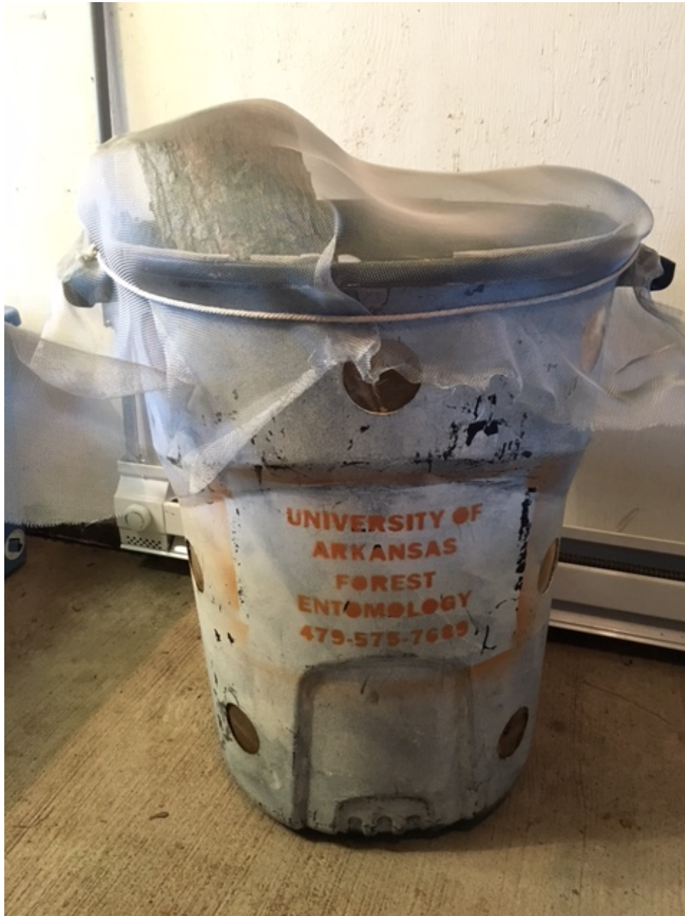
Modified trash can with mesh lid containing experimental shortleaf pine bolt. Used to quarantine and easily check for emerging Monochamus spp.
