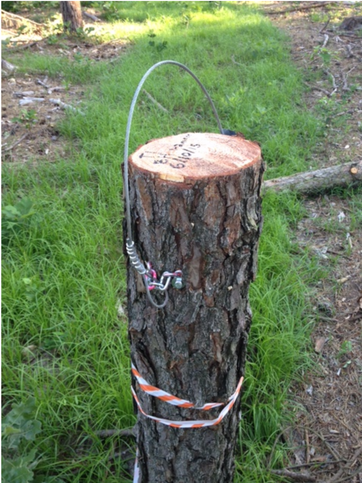
Hardware attached to the top portion of a shortleaf pine bolt. Used for suspending pine bolt in another tree.
