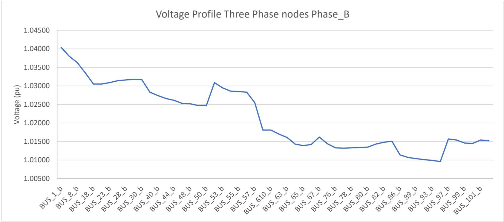
Fig. 3-8. Voltage profile three-phase nodes of phase B.
