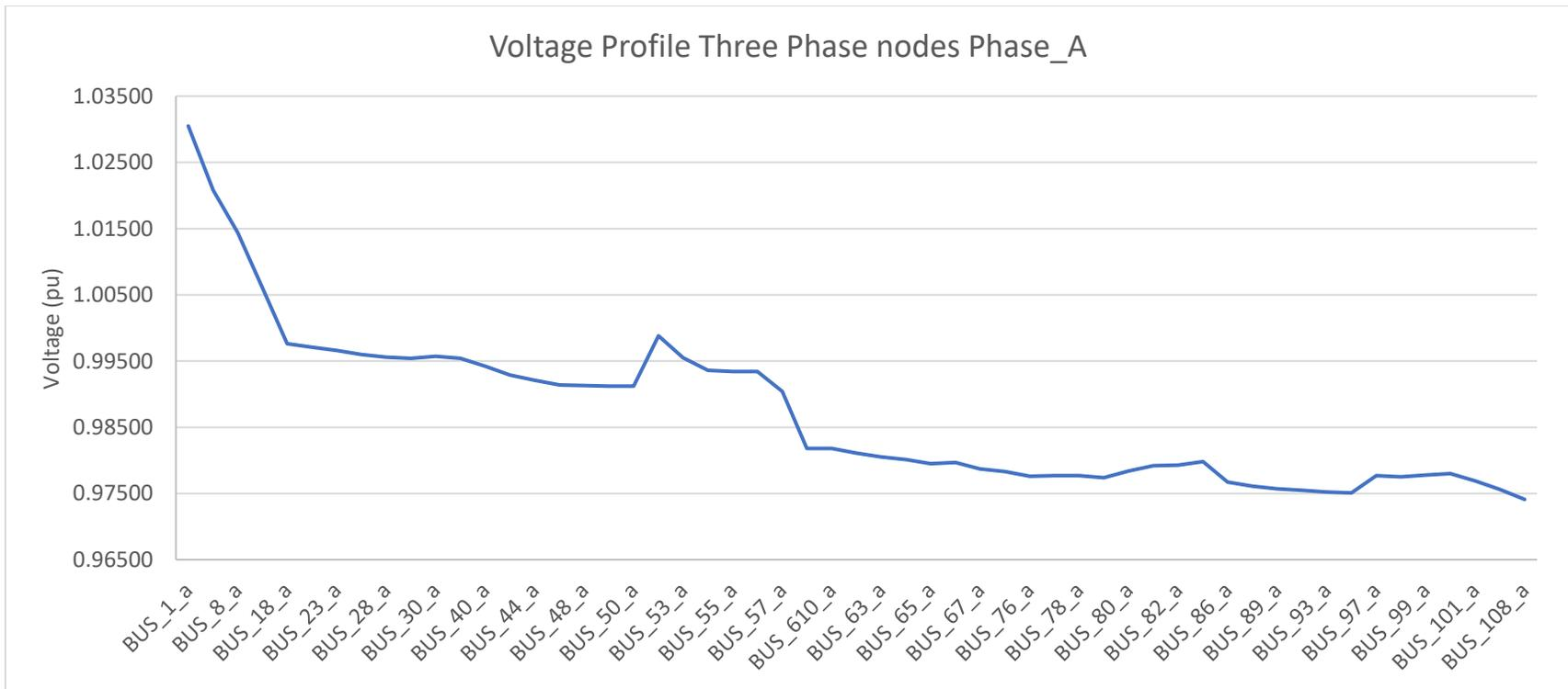
Fig. 3-7. Voltage profile three-phase nodes of phase A.
