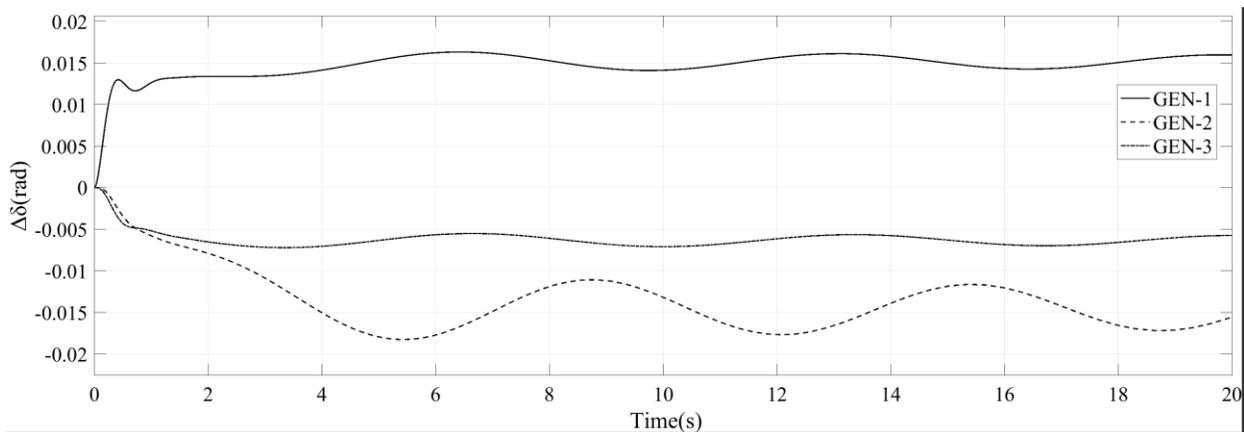
Fig. 4-5. Torque angle ( $\delta$ ) for each generator.
