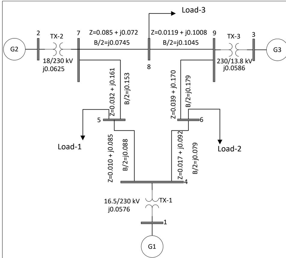
Fig. 4-1. 3-Machine 9-Bus system one line diagram.
