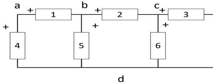
Fig. 3-9. Circuit for node incidence matrix sample.
