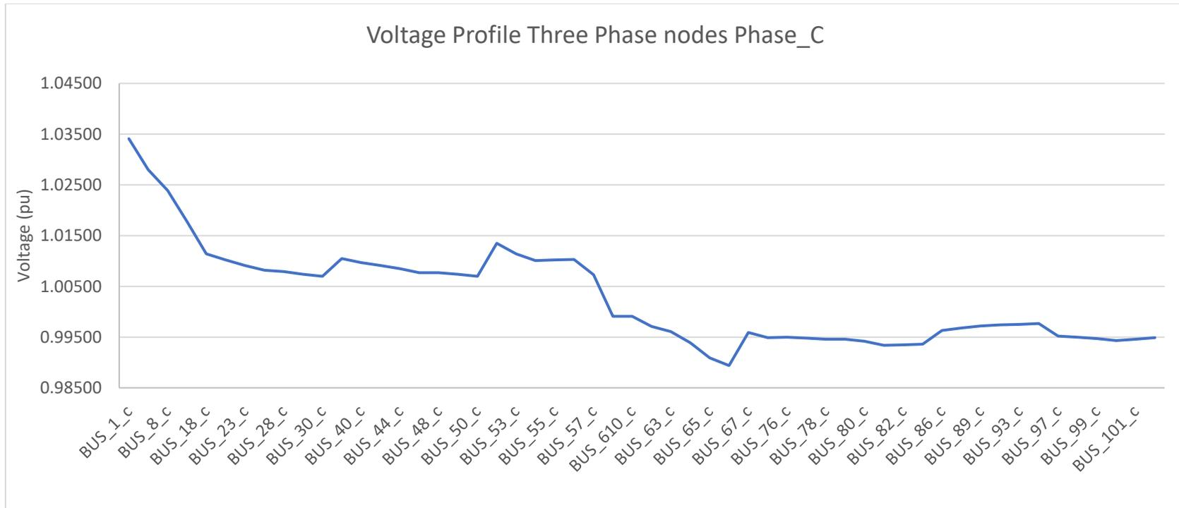
Fig. 3-6. Voltage profile three-phase nodes phase C.
