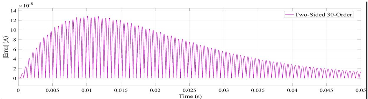
Fig. 3-26. Absolut error of 30-order two-sided reduced system.
