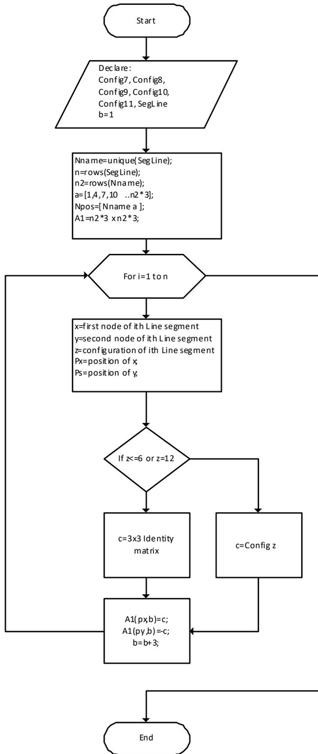
Fig. 3-13. Flow chart of the algorithm for node incident matrix corresponding to line segments.
