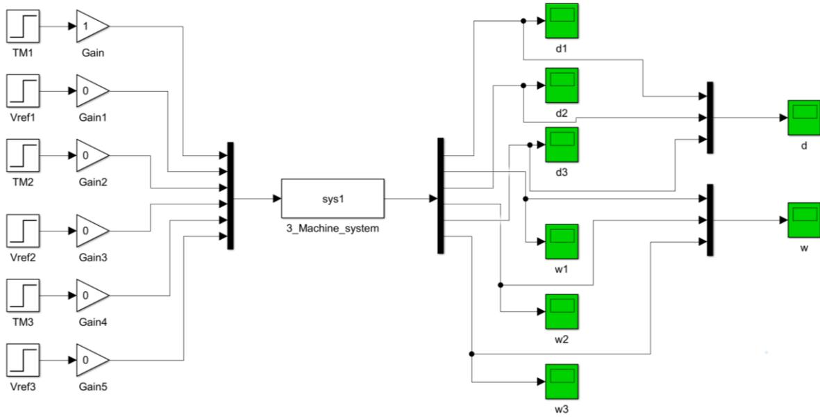
Fig. 4-4. MATLAB/SIMULINK™ simulation set-up for 3-Machine 9-Bus system.
