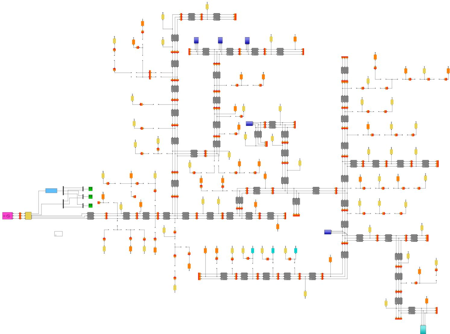
Fig. 3-5. MATLAB/SIMULINK™ model of IEEE-123 Node Test Feeder.
