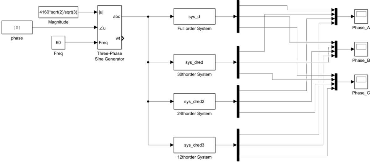
Fig. 3-18. MATLAB/SIMULINK™ setup for comparing reduced models.
