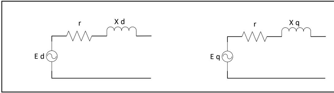
Fig. 4-2. D- and q-axis equivalent two-axis generator model.
