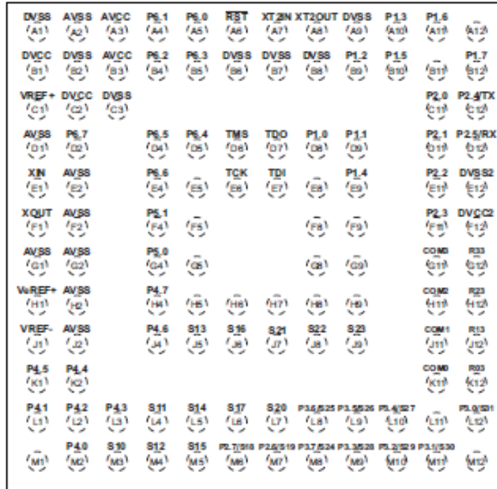
Fig.9 113 ZCA package of MSP430 microcontroller [10]
